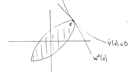
The point  $\sigma$  corresponds to the point on the boundary of the domain of attraction on which V(x) is minimized. We know from Theorem 8 that this will occur at a type-1 equilibrium point. Recall that this means that the Jacobian of (31) evaluated at  $\sigma$  has one right half plane pole, and no poles on the imaginary axis. The stable manifold of  $\sigma$ ,  $W^s(\sigma)$ , is part of  $\partial R_A$ , the boundary of the domain of attraction of the origin.
