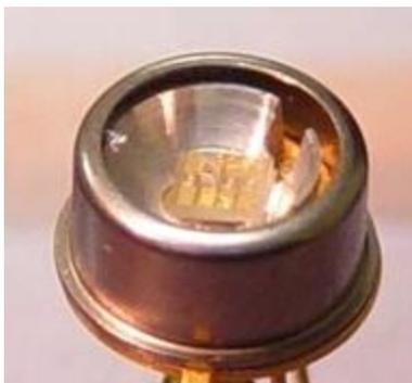
**Figure 2.4. UV LED customized with heat sink, proprietary reflector, transparent windows to optimize the output power from LED (Sensor Electronics)**
