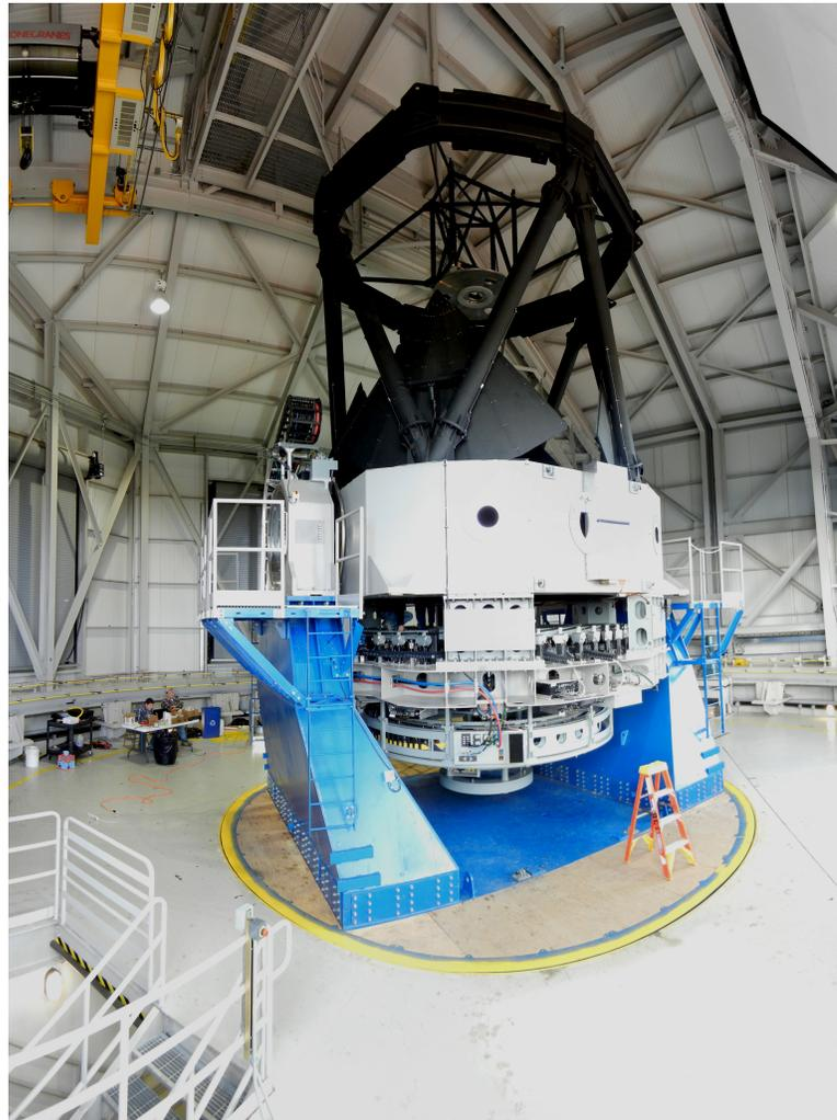
Figure 4.1 The 4.3-meter Discovery Channel Telescope in the stowed position. The instruments sit behind the primary mirror at the base of the telescope in an instrument cube that moves with the telescope. The image was retrieved from <http://www.bu.edu>.
