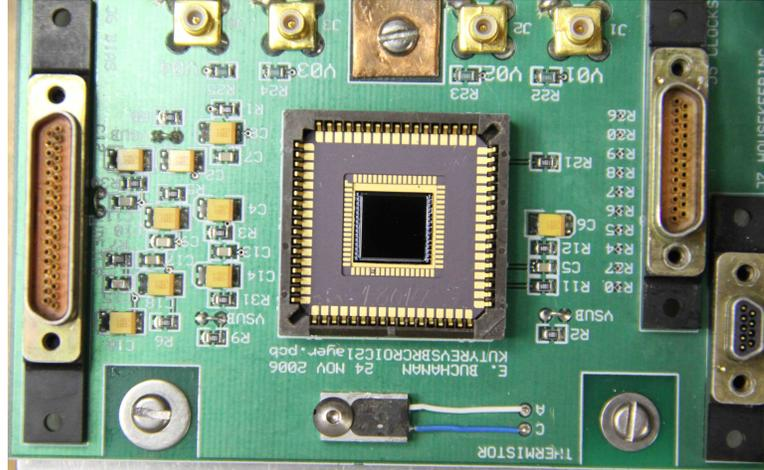
Figure 4.6 RIMAS slit-viewer 256 x 256 pixel InSb detector. Three harnesses connect to the circuit board to deliver clocks and biases to the detector and return the detector signal to the detector acquisition system.
