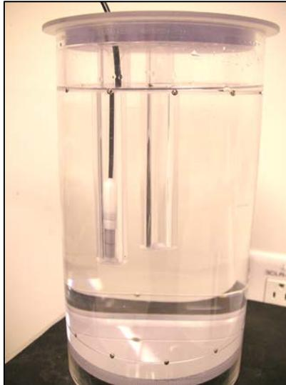
Figure 6.3: Cylindrical phantom with hollow PMMA inserts used for the dose distribution analysis. The Radcal 10x5-0.6 ion chamber is seen here in the peripheral cylinder.
