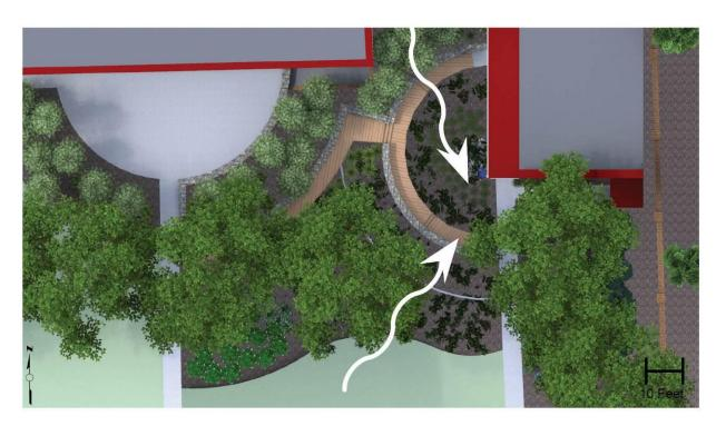
Illustration 4.2: Aerial view of the proposed design with the weir system and elevated decks for water to flow beneath
