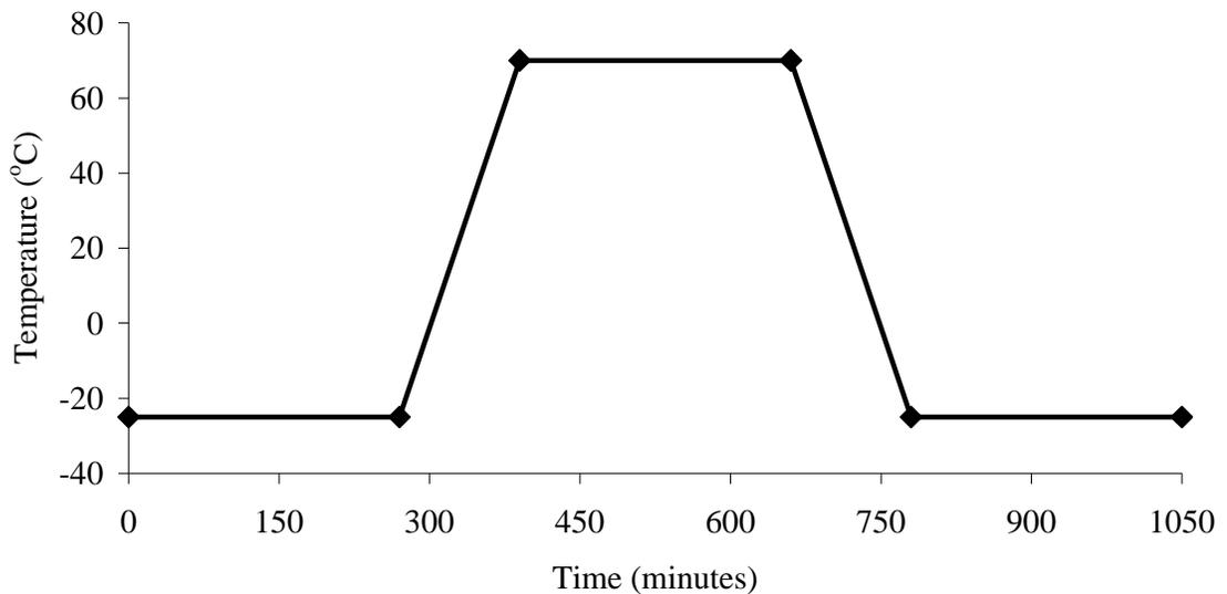
**Figure 4-3 Acceptance temperature cycle**
