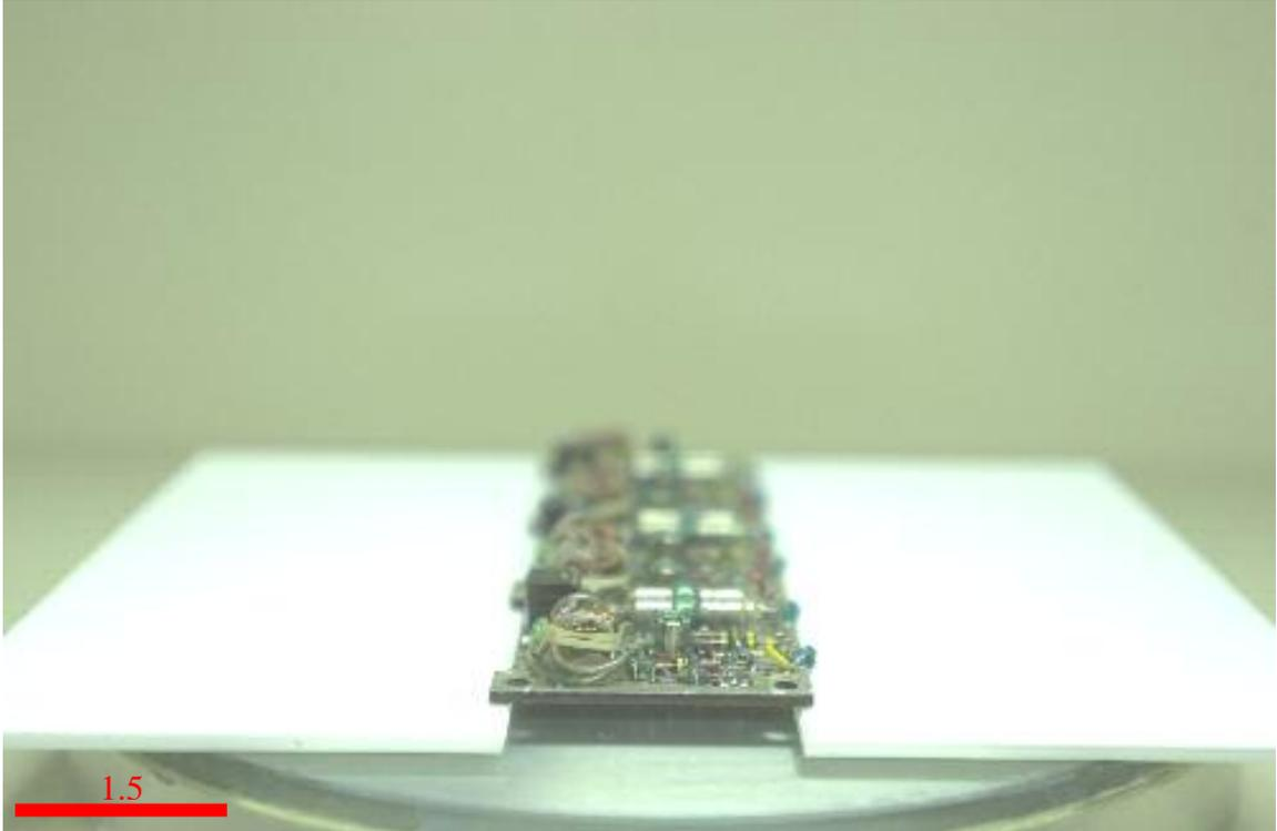
**Figure 3-4:** This photo shows the setup to measure board flatness. The board is suspended by its edges on ceramic plates on a flat glass plate.
