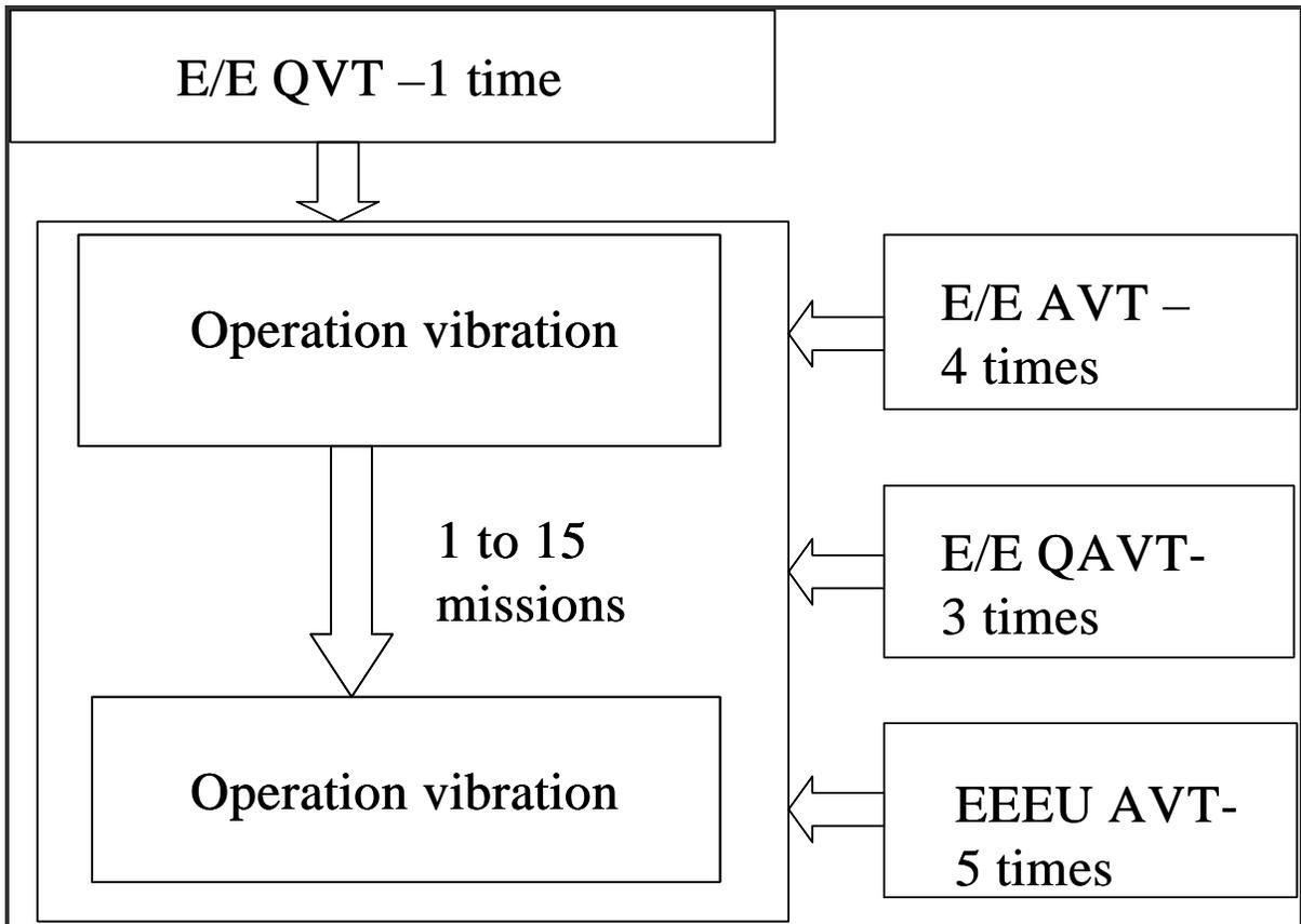
**Figure 4-7: Graphical description of vibration profiles**
