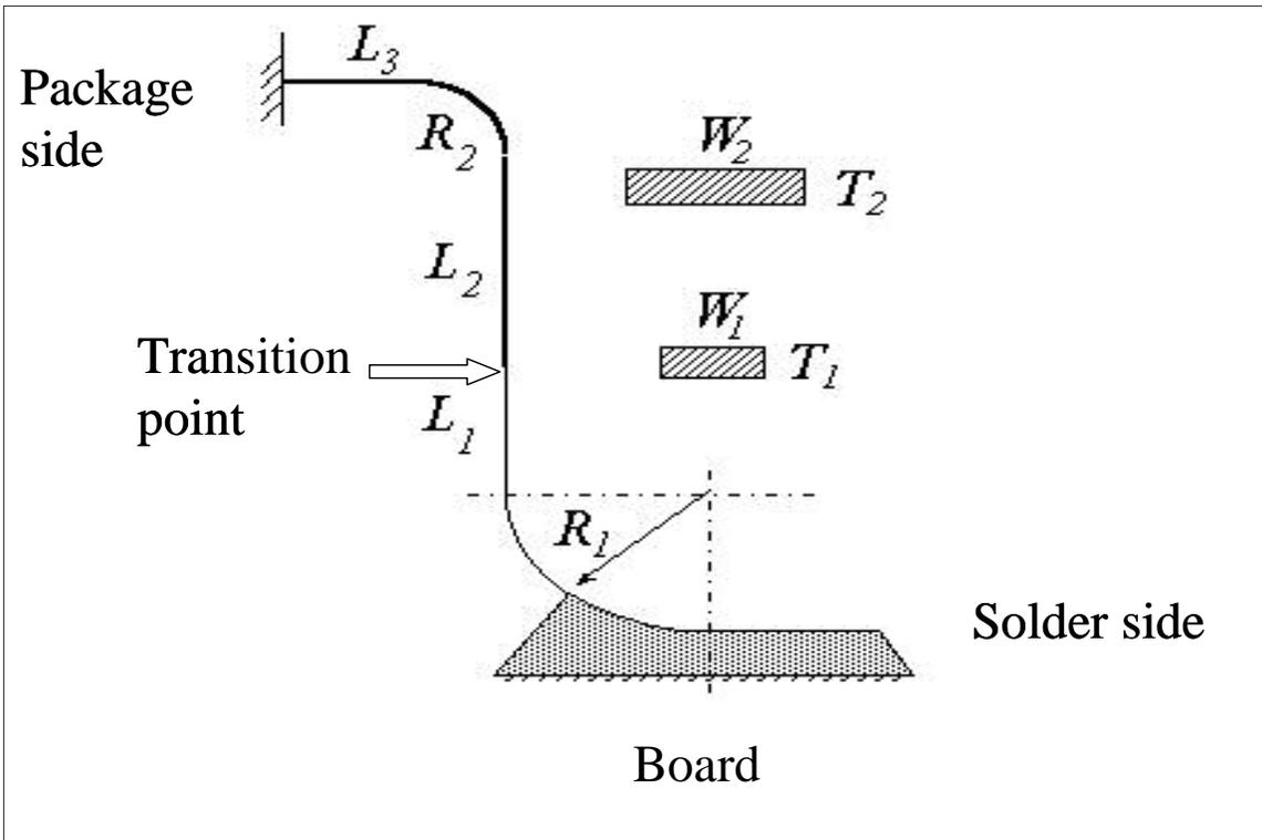
Figure 6-2: Interconnect dimensions for gullwing components
