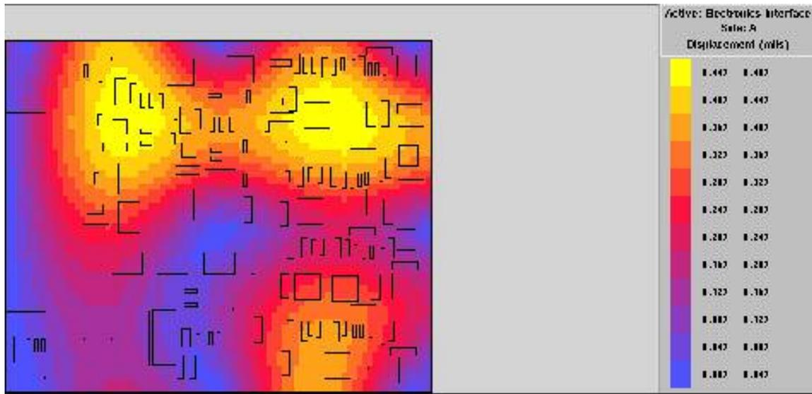
**Figure 6-8: Board displacement due to vibration of Electronics Interface (SPA) board**
