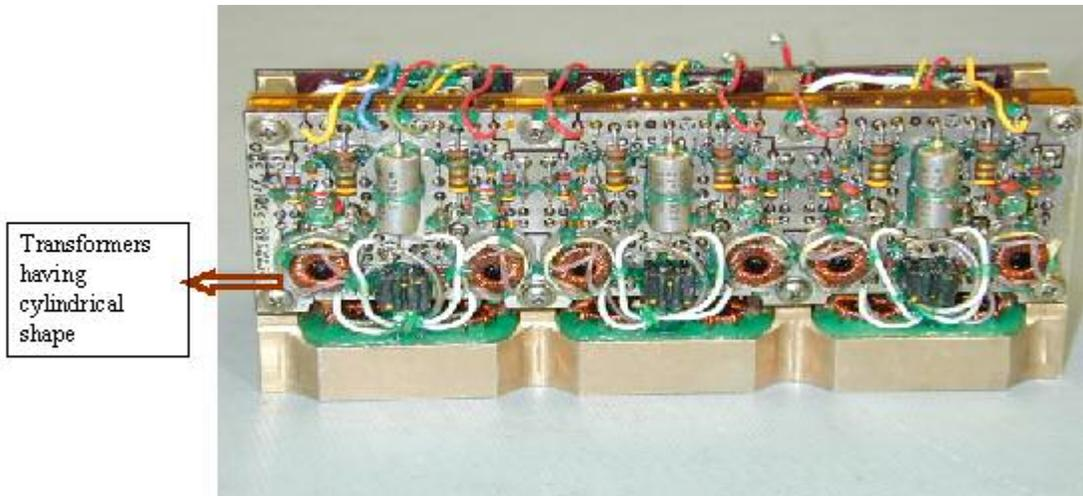
**Figure 6-3: Power Switch Driver Off board**
