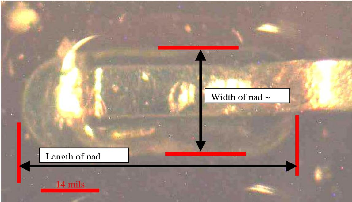
Figure 3-6: This photo shows the length of a pad compared to the width ( $0.08/0.03 \sim 2.7 > 2$ ) which is greater than twice the width, in compliance to the specification.
