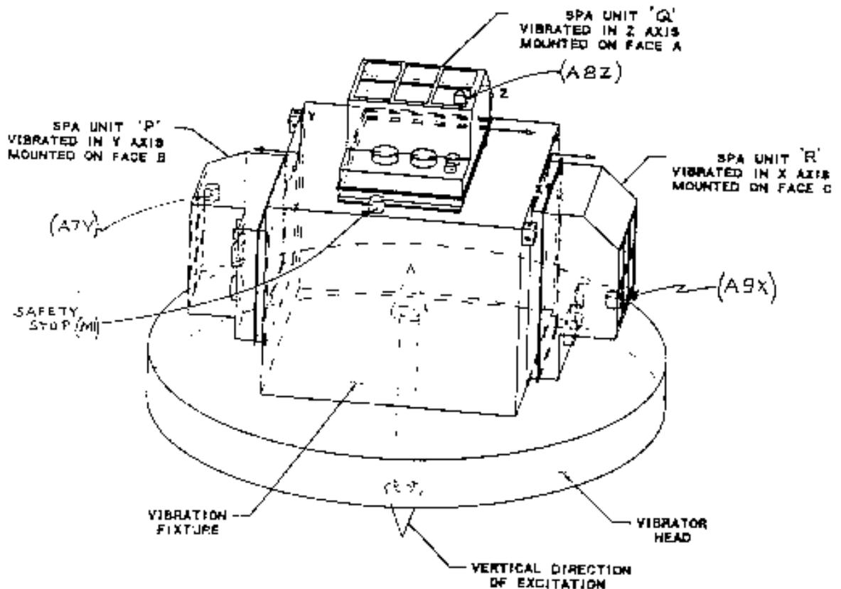
Figure 7-1 : In picture above, the vibration axes are shown for the three SPAs that were vibrated. For the vibration profiles sent, the SPA 212 is on the top of the cube (unit Q / z-axis / face A), SPA 305 is on the left-hand side (unit P / y-axis / face B), and SPA 309 is on the right-hand side (unit R / x-axis / face C).
