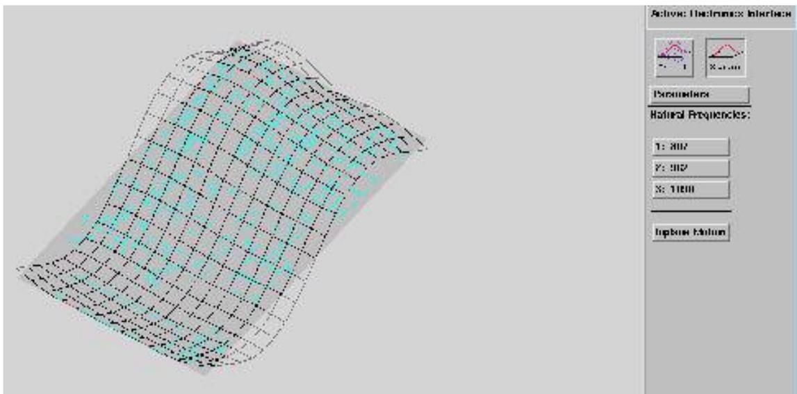
**Figure 6-7: Vibration modes at natural board frequencies (807 Hz) of Electronics Interface (SPA) board**
