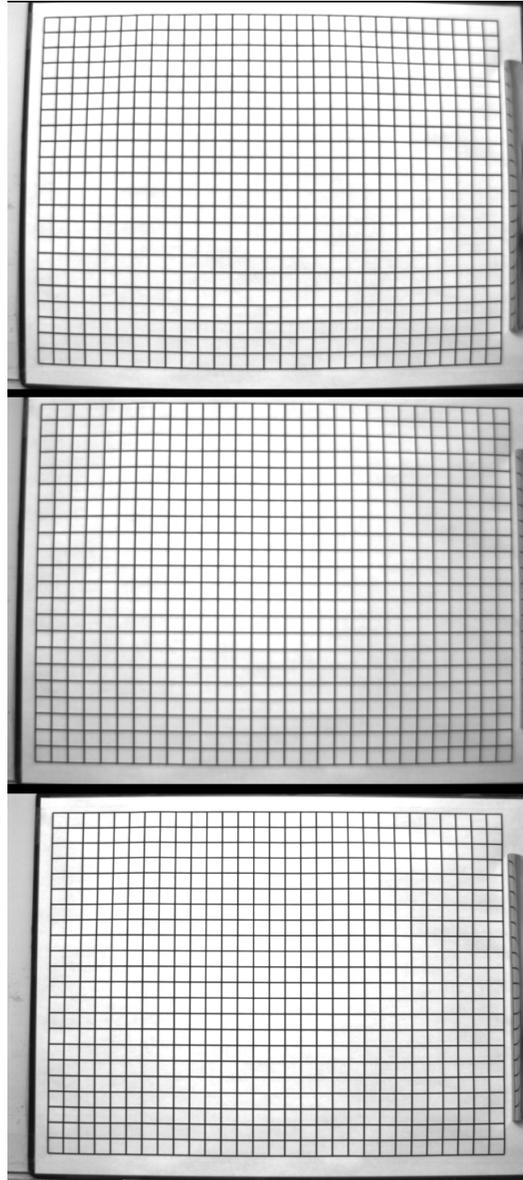
**Fig. 8. Lens distortion analysis. Top: Cosmicar 6 mm, Middle: Canon 7.5 mm, Bottom: Schneider 8 mm.**
