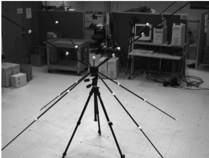
**Fig. 9. Peak Performance calibration frame**
