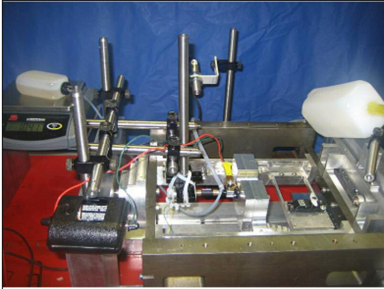
**Figure 1–19: Photograph of a setup used to estimate performance from a Cox 0.16 cc (0.01 cu.in.) displacement model airplane engine [72].**
