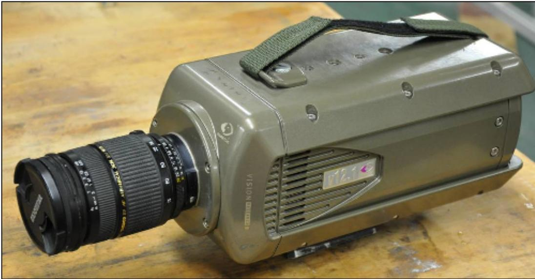
**Figure 6–8: High speed Phantom camera (model v12.1) made by Vision Research Inc. used to acquire combustion images through the quartz window.**
