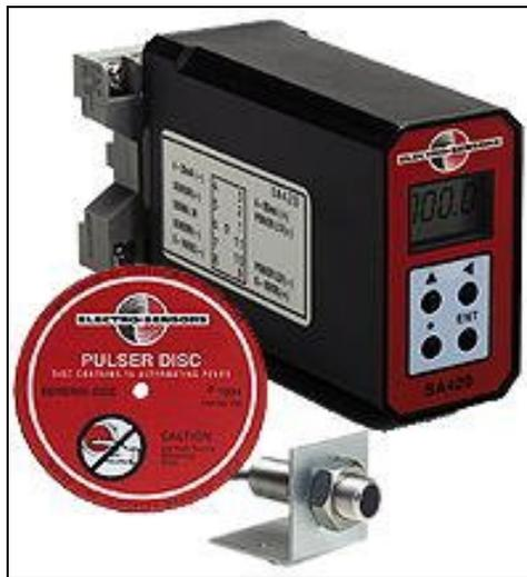
**Figure 2–24: Photograph of the ElectroSensors speed measurement system with the pulser disc, Hall effect sensor and the SA420 signal conditioner.<sup>96</sup>**
