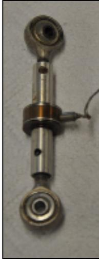
Figure 2–22: Photograph of the Sensotec Model 311AT load cell.
