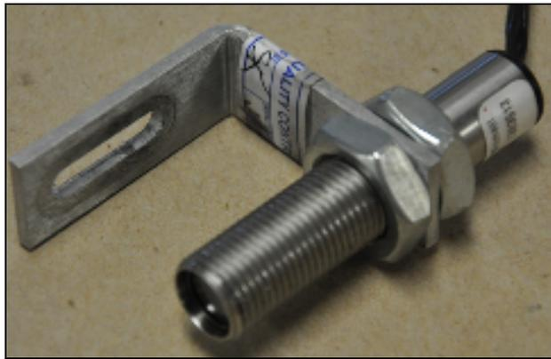
**Figure 2-25: Photograph of the Monarch optical speed sensor.**
