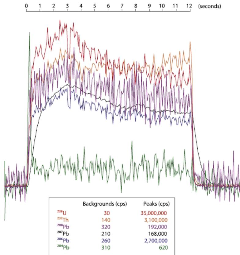
**Figure 3.7** - Example of signal from ablation of a zircon using the LA-ICP-MS at the University of Arizona LaserChron Center. Laser is fired for 12 seconds, with first 3 seconds of data discarded based on rapidly fluctuating signal. Figure from Gehrels et al., 2008.
