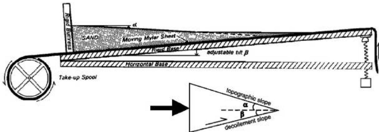
**Figure 1.3** – Original model developed by Davis et al. (1983) that used sand and a moving mylar sheet to approximate wedge formation. Lower schematic shows an idealized critical taper (Horton, 1999).
