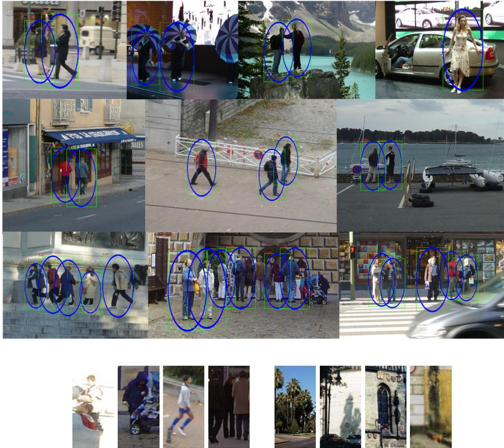
Figure 2.13: Detection results. Top: Example detections on the INRIA test images, nearby windows are merged based on distances; Bottom: Examples of false negatives (FNs) and false positives (FPs) generated by our detector.
