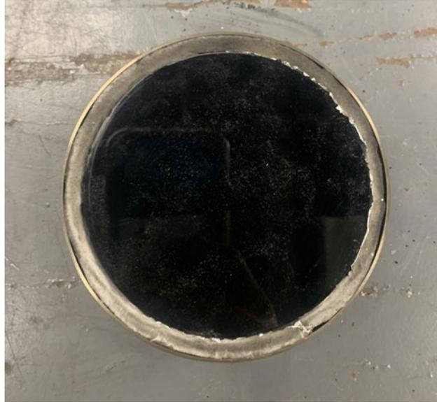
**Figure 4-1. Picture of PMMA sample used in FPA burn test.**
