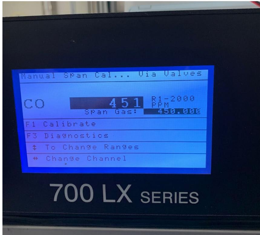
**Figure A-5. Picture of analyzer screen after Step 11.**
