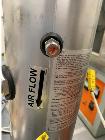
**Figure 2-10, Picture of Thermocouple port**
