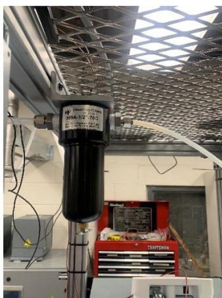
Figure 2-14. Picture of FPA soot filter.
