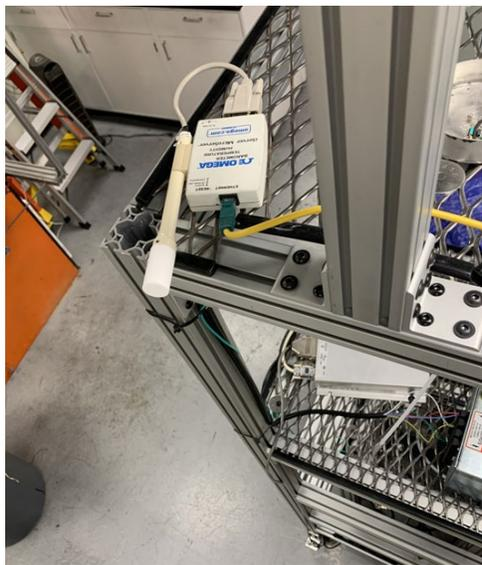
**Figure 2-21. Picture of barometric pressure/absolute temperature/absolute humidity probe.**
