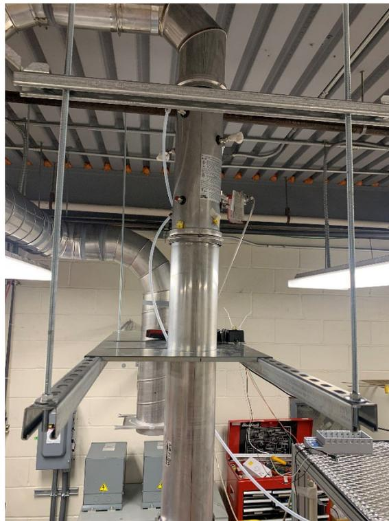
**Figure 2-7. Picture of mixing section and test section installed.**
