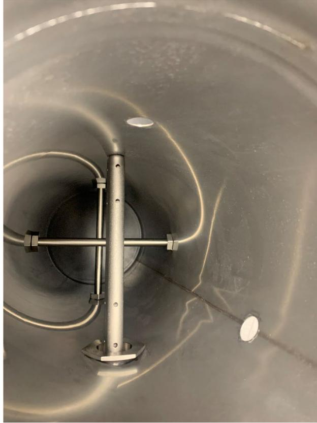
**Figure 2-11. Picture of inside of testing section with the pitot tube installed.**
