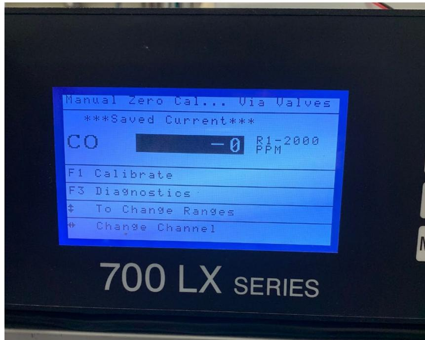
**Figure A-3. Picture of analyzer screen after Step 6.**
