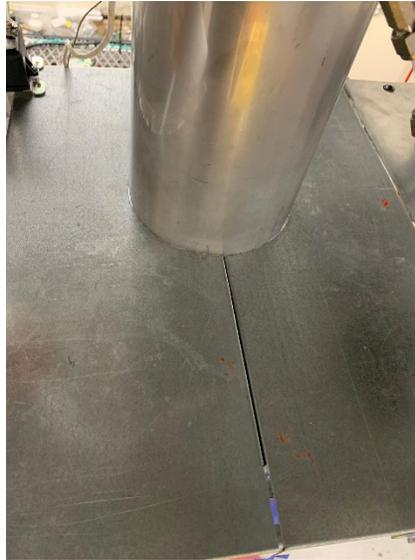
**Figure 2-6. Picture of steel plates clamping the duct fixture in place.**
