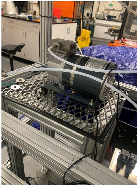
**Figure 2-16. Picture of sample pump for FPA.**
