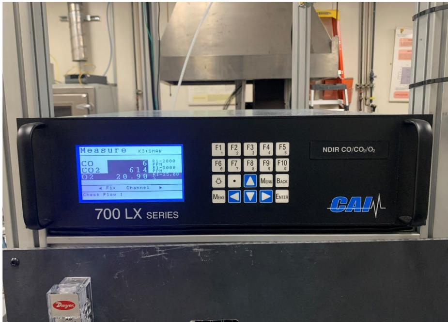
Figure 2-19. Picture of CO/CO<sub>2</sub>/O<sub>2</sub> analyzer.
