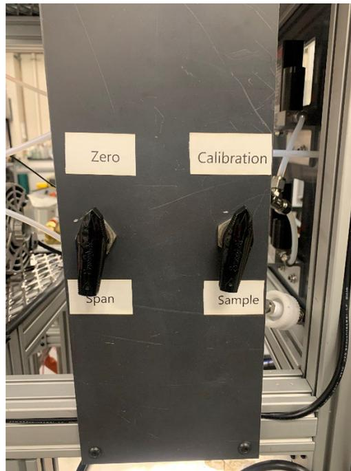
**Figure A-1. Ball valves on calibration panel in correct orientation for zero calibration.**
