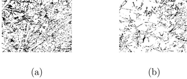
Figure 4.3: (a) Black-white image obtained by thresholding intensity values between 100 and 120, its box-counting fractal dimension  $D = 1.67$ . (b) Black-white image obtained by thresholding intensity values between 80 and 100, its box-counting fractal dimension  $D = 1.49$ .
