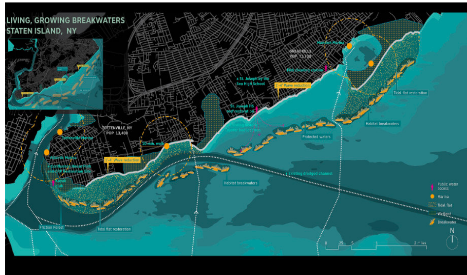
Figure 24: Living Breakwaters Project along the East and South Shore of Staten Island plans to develop a breakwater that grows with the ecological environment while protecting the shoreline. 2014. http://www.rebuildbydesign.org/project/scape-landscape-architecture-final-proposal/ .
