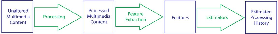
Figure 3.1: Typical process that a multimedia signal may go through when considering forensics.
