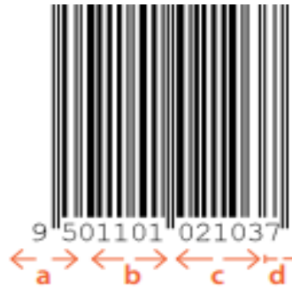
Figure 3.2 - GTIN Barcode Structure for a one dimensional barcode a) GS1 Prefix, b) Company Number, c) Item Reference Number, d) Check Digit (GS1, 2012).
