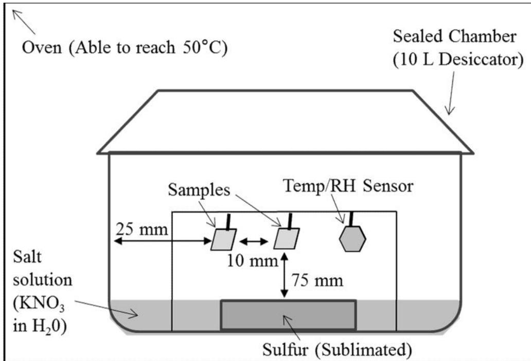
**Figure 6. Schematic of the Flowers of Sulfur Test**
