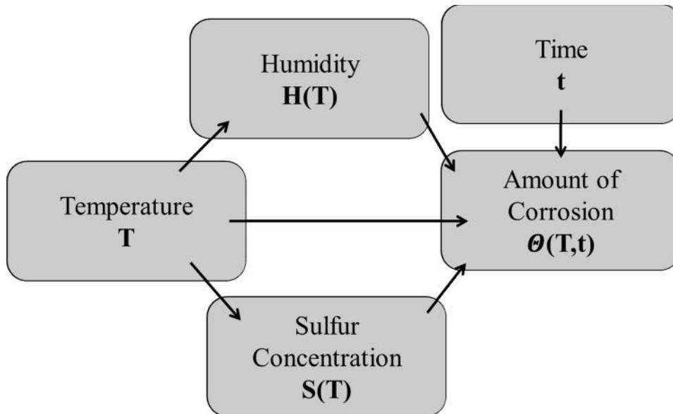
**Figure 13. Factors contributing to corrosion in the FOS**
