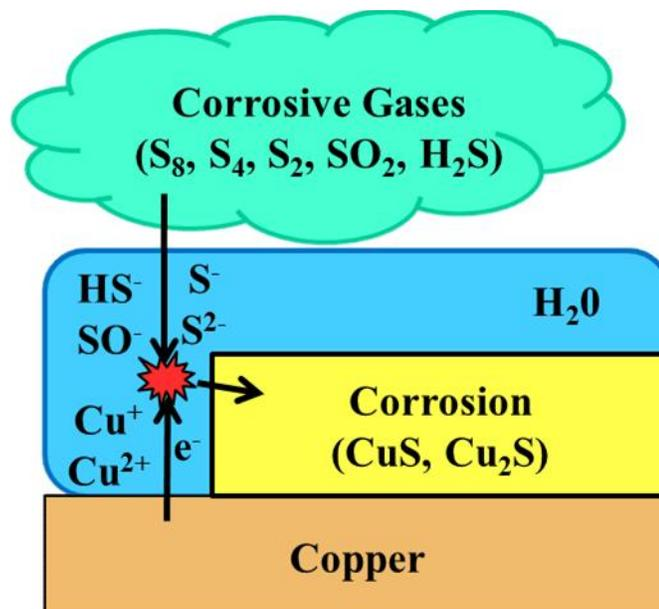
**Figure 2. Copper corrosion in a sulfur-containing atmosphere**
