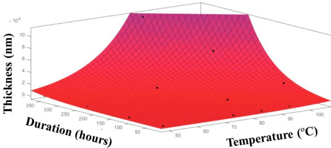
**Figure 26. Model for film thickness as a function of time and temperature**
