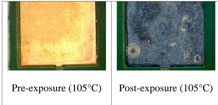
**Figure 29. ImAg boards in high temperature FOS tests**
