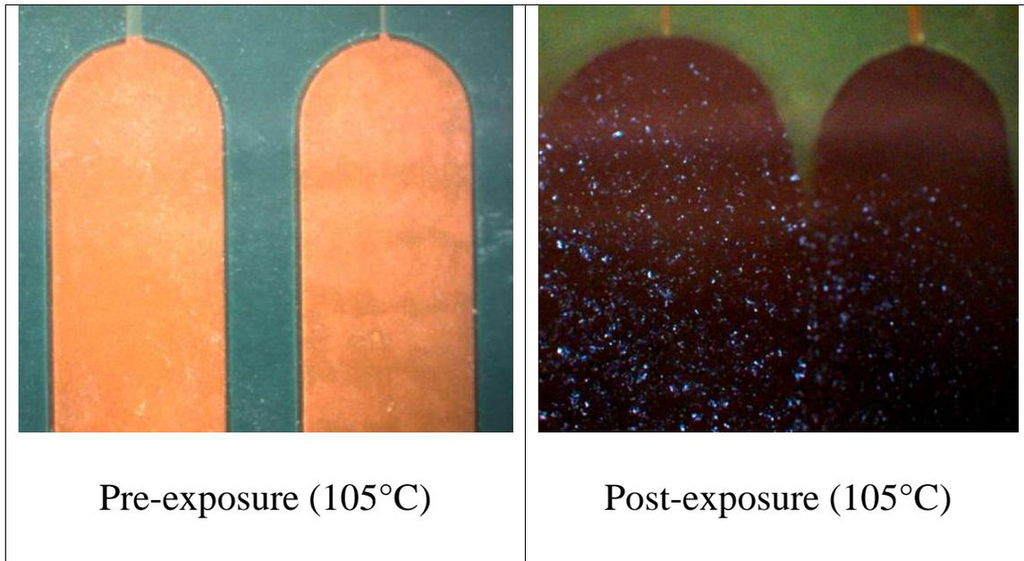
**Figure 30. OSP boards in high temperature FOS tests**
