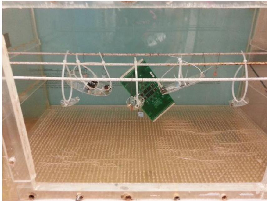
**Figure 5. Samples in the MFG chamber at CALCE**
