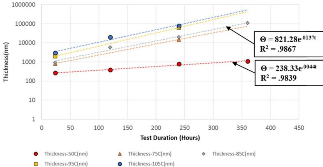
**Figure 23. Corrosion Film Thickness as an exponential function of time.**
