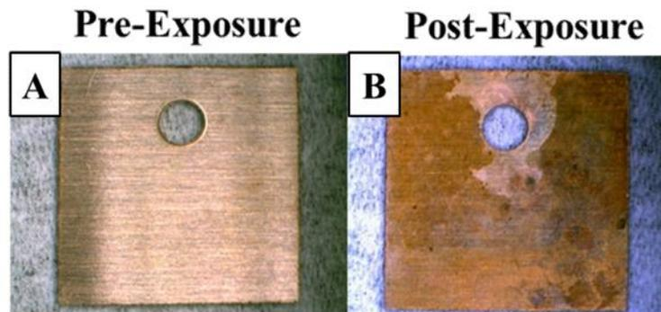
**Figure 1. Copper coupon before (A) and after (B) a corrosive**
