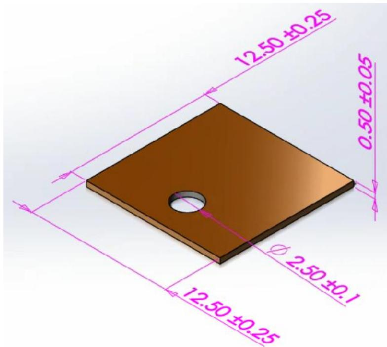
**Figure 16. Copper coupon Schematic (Dimensions in mm)**
