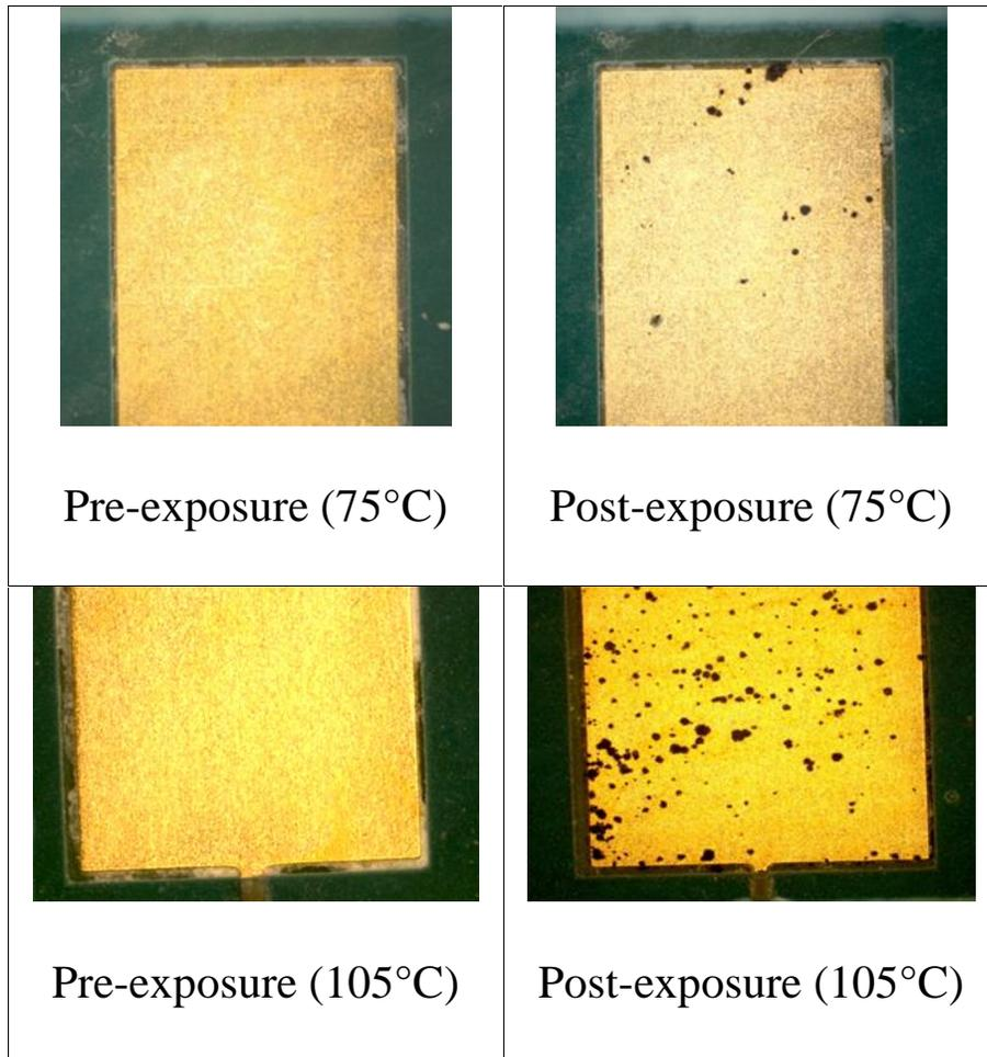
**Figure 28. ENEPIG boards in high temperature FOS tests**
