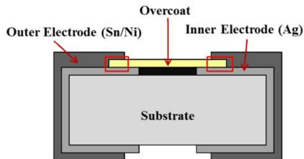
**Figure 11. Chip resistor (Failure sites highlighted)**
