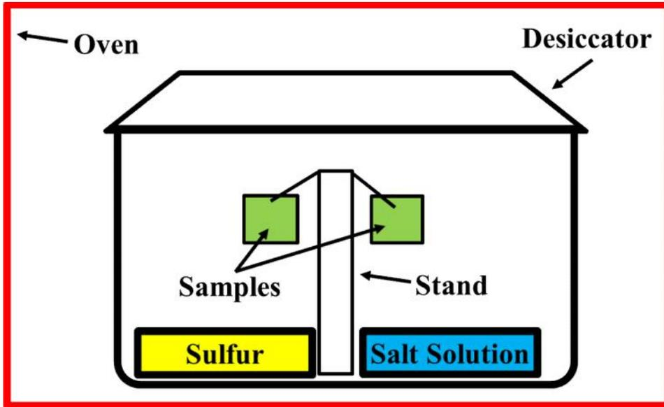
**Figure 32. Flowers of Sulfur Test Schematic**
