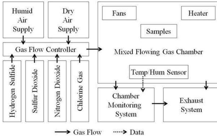
**Figure 4. Schematic of the MFG Test**
