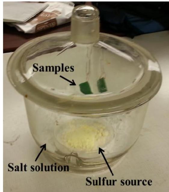
**Figure 7. Picture of the ASTM-B809 FOS Test setup**
