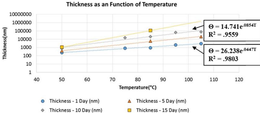
**Figure 21. Corrosion Film Thickness as a Function of Temperature**
