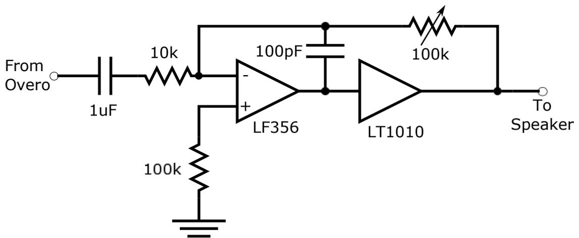
Figure 3.5: Circuit for powering speakers. The LT1010 is an integrated circuit specifically designed to allow op-amps to drive reactive loads, like the piezoelectric speakers we used.
