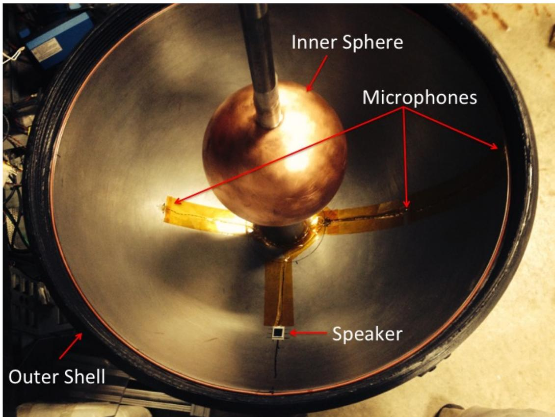
Figure 3.4: Photograph of bottom hemisphere with inner sphere, microphones, and speaker installed.
