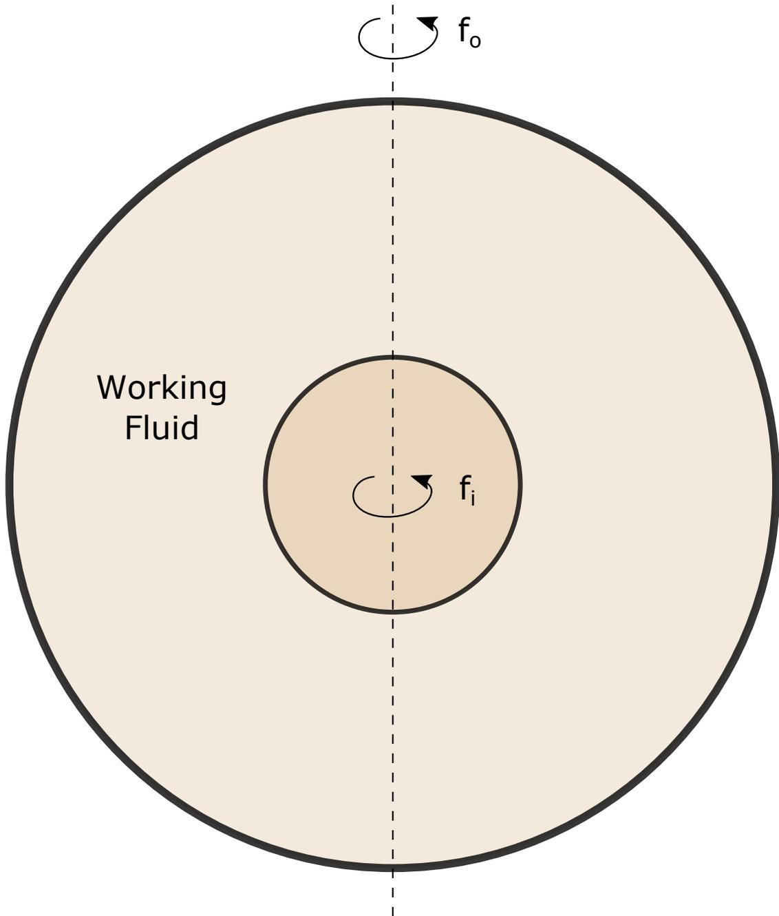
Figure 1.1: Diagram of Spherical Couette Flow. The working fluid is located between an outer spherical shell and an inner sphere; flow is driven by differential rotation of the inner and outer spheres, which share an axis. For experimental devices, the inner sphere must be supported by a shaft arrangement.
