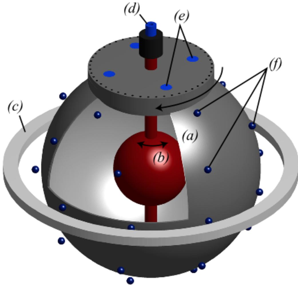
Figure 3.8: Instrumentation for 3 m Experiment. (a) Outer spherical shell; (b) Inner sphere; (c) External magnet, located around the vessel's equator; Note that in later experiments a pair of external magnets was used, with the magnets located symmetrically above and below the equator; (d) Reaction torque sensor; (e) Instrumentation ports; (f) External Hall effect magnetic field probes. Originally Figure 1 from [90].
