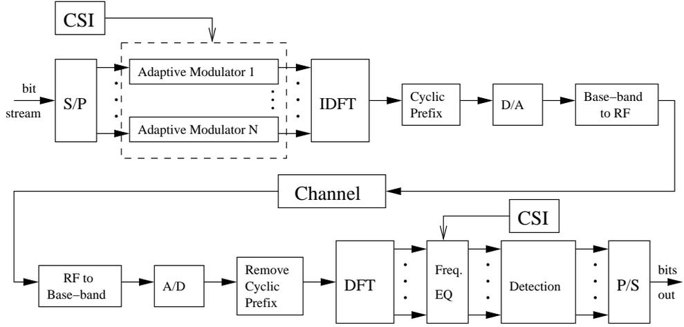
Figure 1.2: Single-user OFDM transmitter and receiver.
