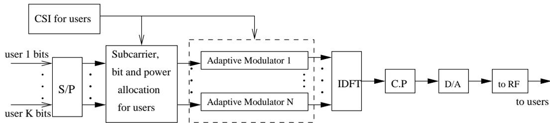
Figure 2.1: Multi-user OFDM transmitter diagram.
