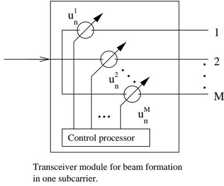
Figure 1.4: A transceiver module that forms one beam.
