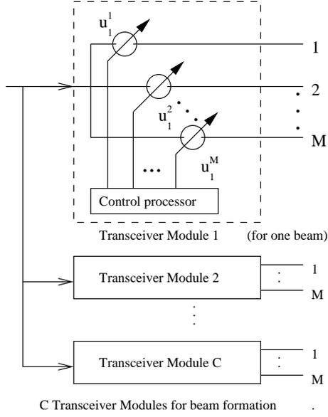
Figure 6.2: The structure of  $C$  transceiver modules.
