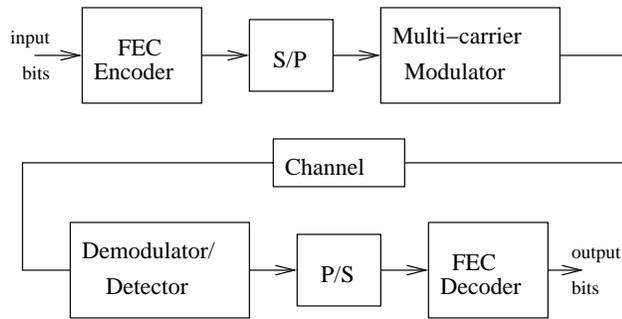
Figure 4.1: Schematic diagram of an OFDM transmission system with FEC encoding.
