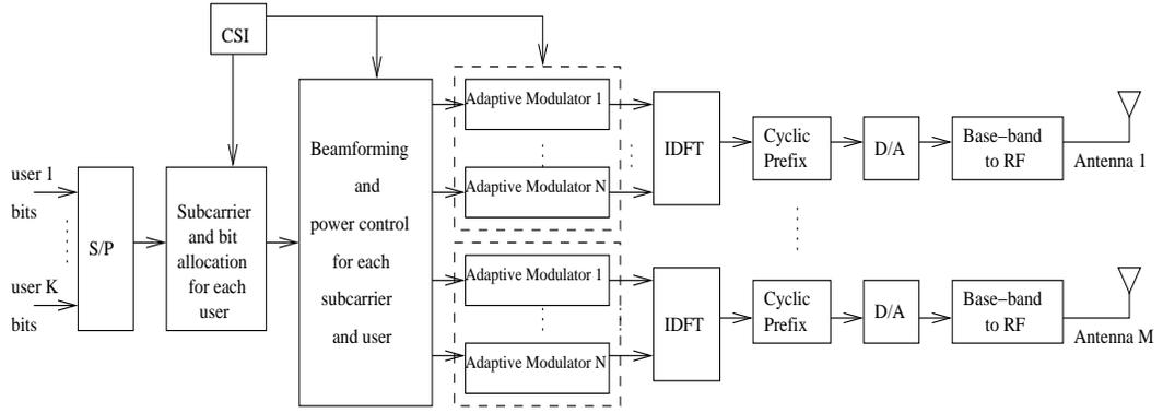
Figure 5.1: Block diagram of a multi-user OFDM/SDMA transmitter.
