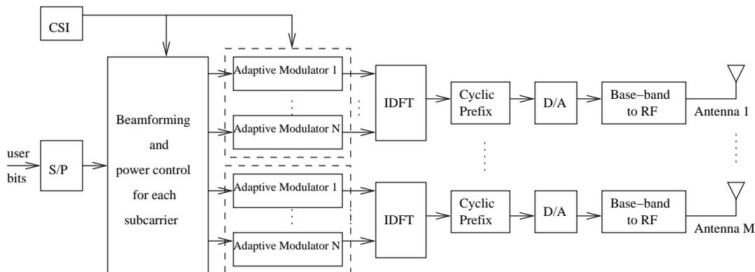
Figure 1.3: Single-user OFDM/SDMA transmitter.
