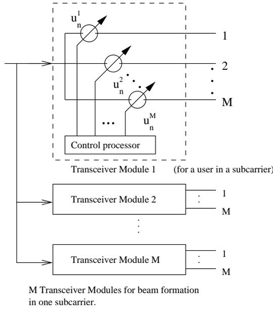
Figure 5.2: The structure of  $M$  transceiver modules for one subcarrier,  $n$ .
