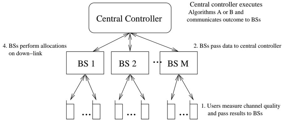
Figure 2.2: Schematic diagram for implementation of algorithms A and B.
