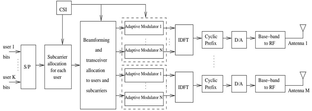
Figure 6.1: Block diagram of a multi-user OFDM/SDMA transmitter with limited transceiver resources.
