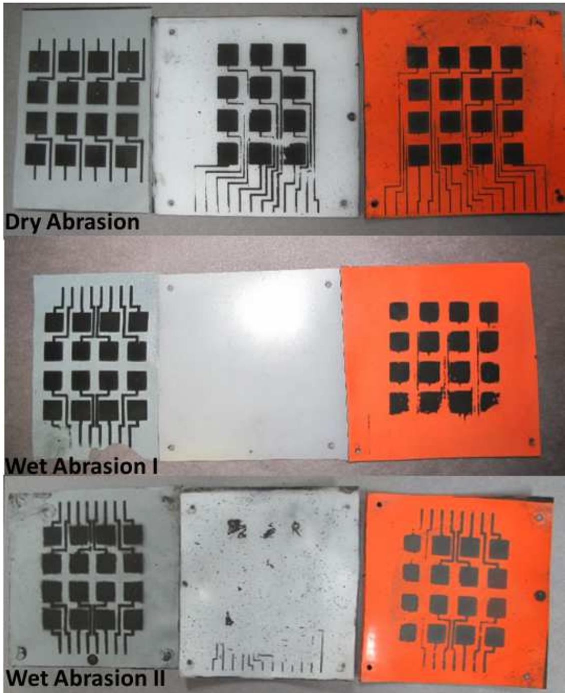
Figure 3.21: Sample set of materials from differing abrasion tests
