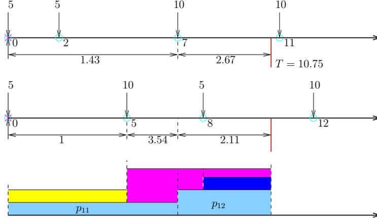
Figure 7.10: Optimal transmit powers  $\mathbf{p}_1 = [1.43, 1.43, 2.67]$  mW,  $\mathbf{p}_2 = [1, 3.54, 2.11]$  mW, with durations  $\mathbf{l} = [5, 2, 3.75]$  s.
