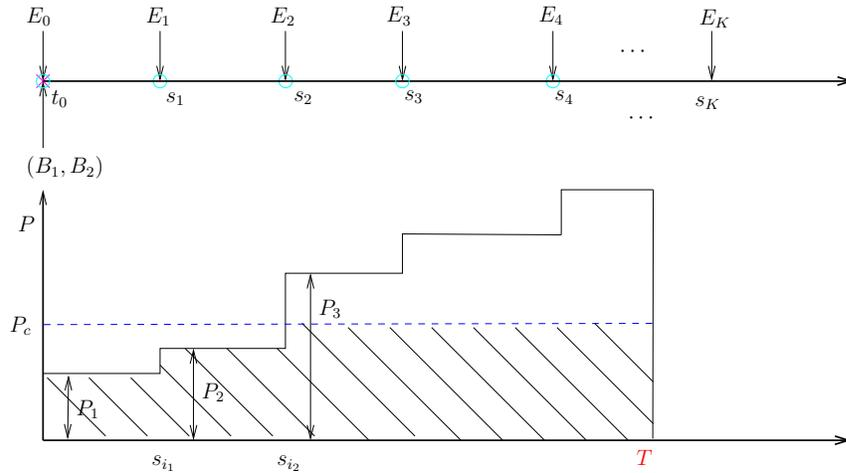
Figure 6.7: Optimally splitting total power between the signals that go to the two users.
