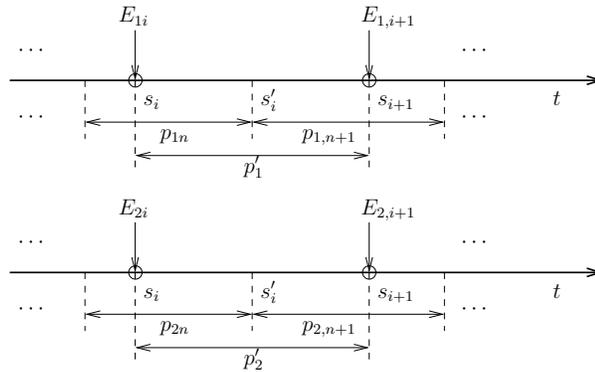
Figure 7.3: The power/rate must remain constant between energy harvests.
