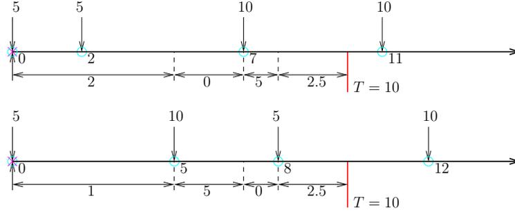
Figure 7.9: Optimal transmit powers  $\mathbf{p}_1 = [2, 0, 5, 2.5]$  mW,  $\mathbf{p}_2 = [1, 5, 0, 2.5]$  mW, with durations  $\mathbf{l} = [5, 2, 1, 2]$  s.
