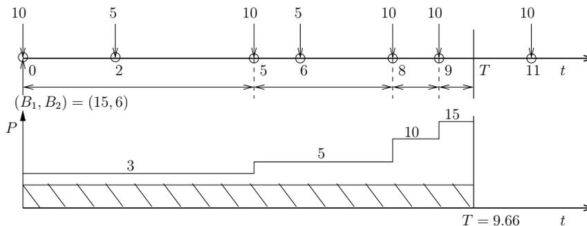
Figure 6.11: Cut-off power  $P_c = 1.933$  mW. Optimal transmit rates are  $r_1 = 1.552$  Mbps,  $\mathbf{r}_2 = [0.274, 0.680, 1.369, 1.834]$  Mbps, with durations  $\mathbf{l} = [5, 3, 1, 0.66]$  s.
