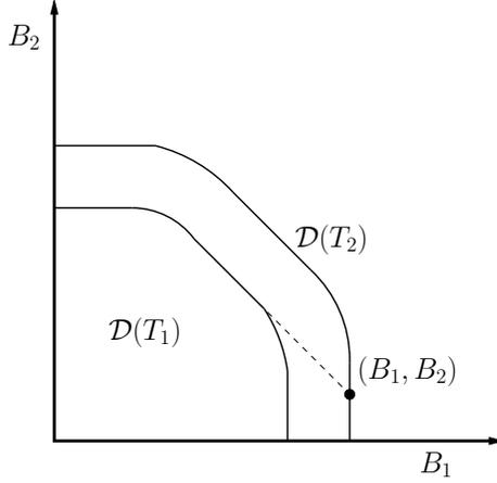
Figure 7.7: The minimum transmission completion time  $T$  to depart  $(B_1, B_2)$ .
