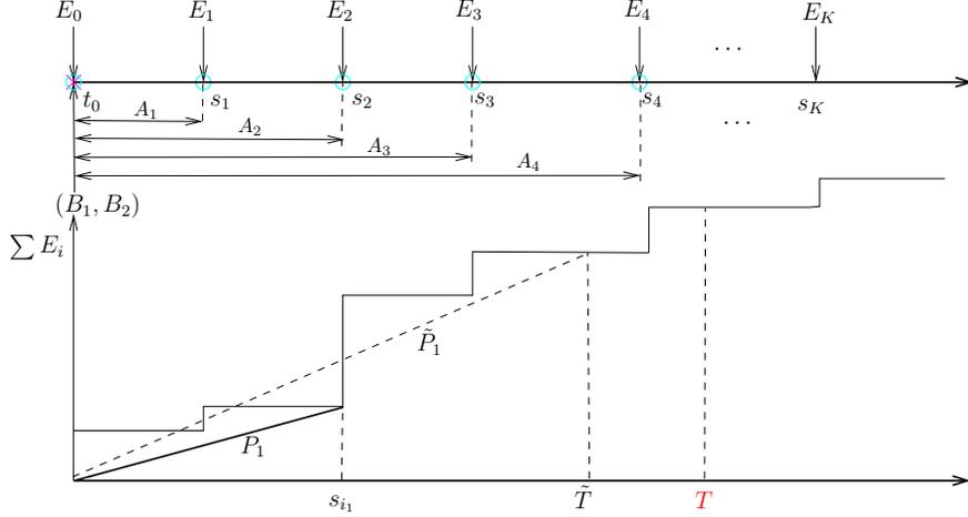
Figure 6.8: Determining the optimal total power level of the first epoch.
