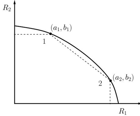
Figure 4.1: The asymmetric pentagon rate region with a non- $45^\circ$  dominant face. Corner point 2 has larger sum-rate, i.e.,  $a_2 + b_2 > a_1 + b_1$ .
