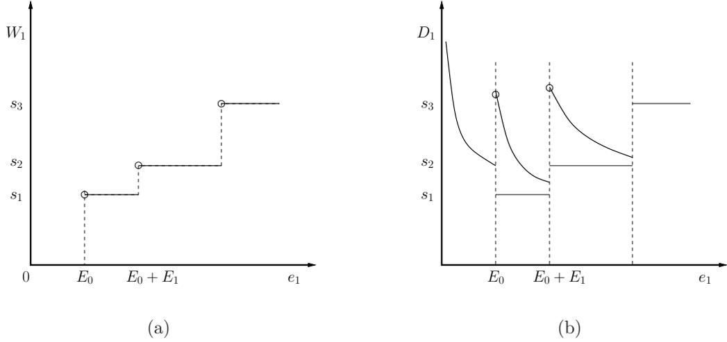
Figure 8.7: (a) The waiting time for the first packet,  $W_1$  and (b) the delay for the first packet,  $D_1$ .
