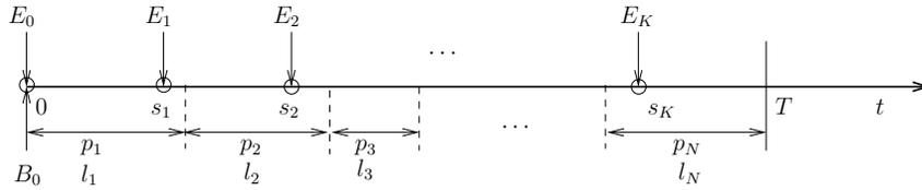
Figure 5.4: The sequence of transmission powers and durations.
