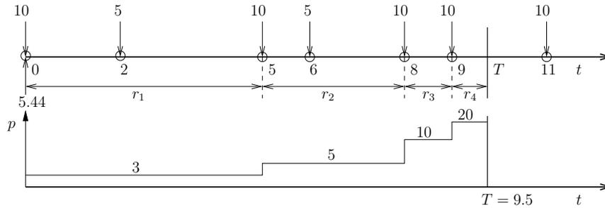
Figure 5.9: Optimal transmit powers  $\mathbf{p} = [3, 5, 10, 20]$  mW, with durations  $\mathbf{l} = [5, 3, 1, 0.5]$  s.
