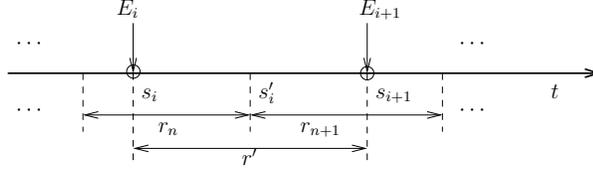
Figure 5.5: The rate must remain constant between energy harvests.
