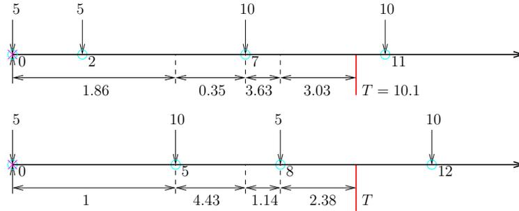
Figure 7.11: Optimal transmit powers  $\mathbf{p}_1 = [1.86, 0.35, 3.63, 3.03]$  mW,  $\mathbf{p}_2 = [1, 4.43, 1.14, 2.38]$  mW, with durations  $\mathbf{l} = [5, 2, 1, 2.1]$  s.
