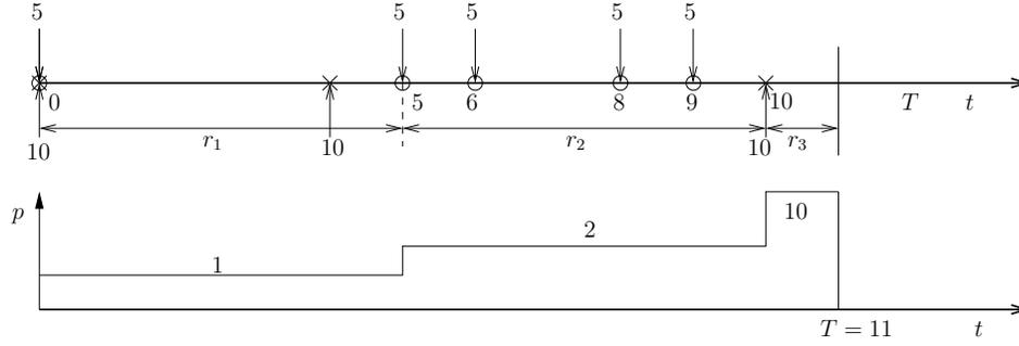
Figure 5.10: Optimal transmit powers  $\mathbf{p} = [1, 2, 10]$  mW, with durations  $\mathbf{l} = [5, 5, 1] \times 10^{-2}$  s.
