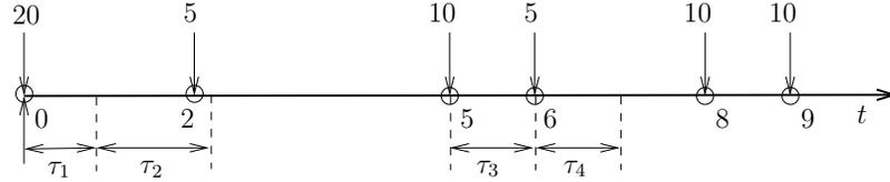
Figure 8.12: The optimal energy allocation  $\mathbf{e} = [10.5, 9.5, 10, 10] \times 10^{-2}$  mJ, with duration  $\boldsymbol{\tau} = [0.89, 1.15, 1, 1] \times 10^{-2}$  s, respectively.
