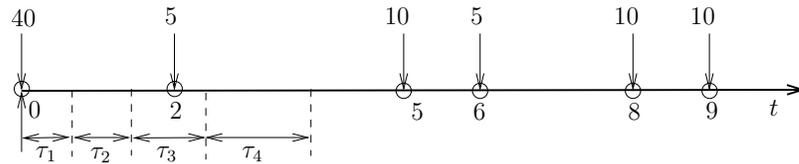
Figure 8.13: The optimal energy allocation  $\mathbf{e} = [12.6, 11.8, 10.9, 9.7] \times 10^{-2}$  mJ, with duration  $\boldsymbol{\tau} = [0.63, 0.70, 0.82, 1.07] \times 10^{-2}$  s, respectively.
