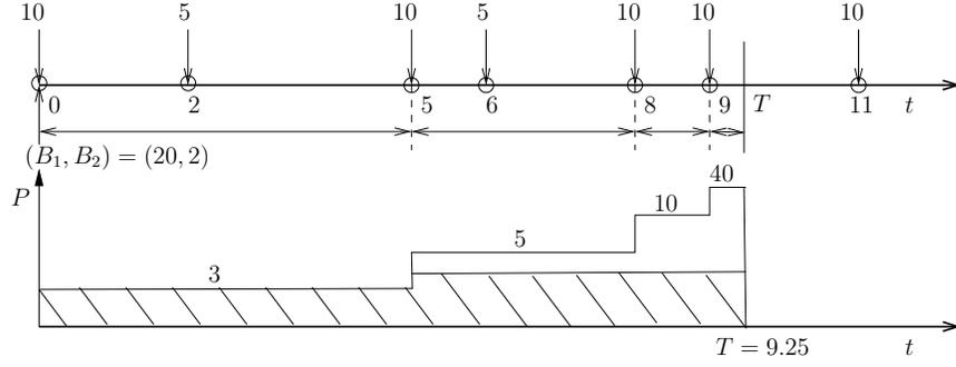
Figure 6.12: Cut-off power  $P_c = 4.107$  mW. Optimal transmit rates  $\mathbf{r}_1 = [2, 2.353, 2.353, 2.353]$  Mbps and  $\mathbf{r}_2 = [0, 0.167, 0.856, 2.570]$  Mbps, with durations  $\mathbf{l} = [5, 3, 1, 0.25]$  s.
