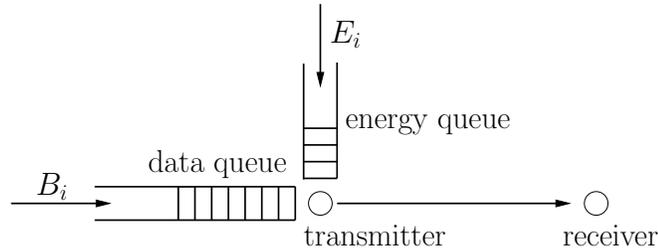
Figure 5.1: An energy harvesting communication system model.
