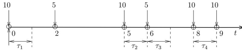
Figure 8.11: The optimal energy allocation  $\mathbf{e} = [10, 10, 10, 10] \times 10^{-2}$  mJ, with duration  $\boldsymbol{\tau} = [1, 1, 1, 1] \times 10^{-2}$  s, respectively.
