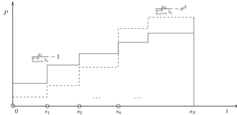
Figure 6.6: The value of the optimal transmit power is always equal to the curve on top.
