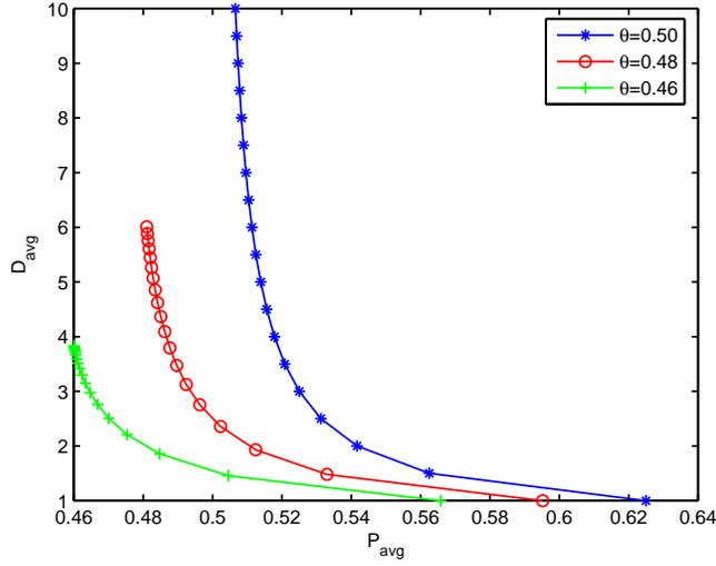
Figure 2.6: The average delay versus average power in the symmetric scenario.
