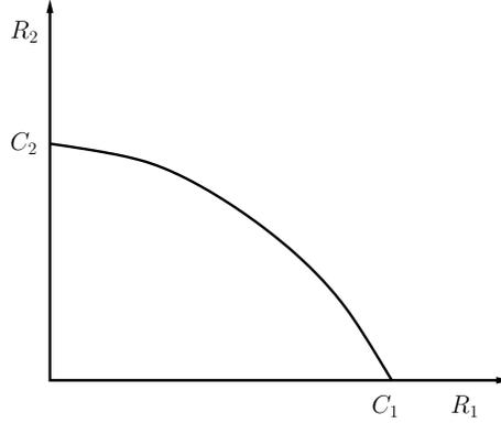
Figure 6.3: The capacity region of the two-user AWGN broadcast channel.
