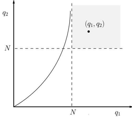
Figure 4.5: The switch curve of the discounted-cost MDP.
