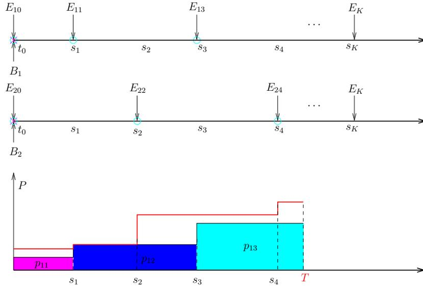
Figure 7.6: The optimal transmit power for the second user to maximize its departure.
