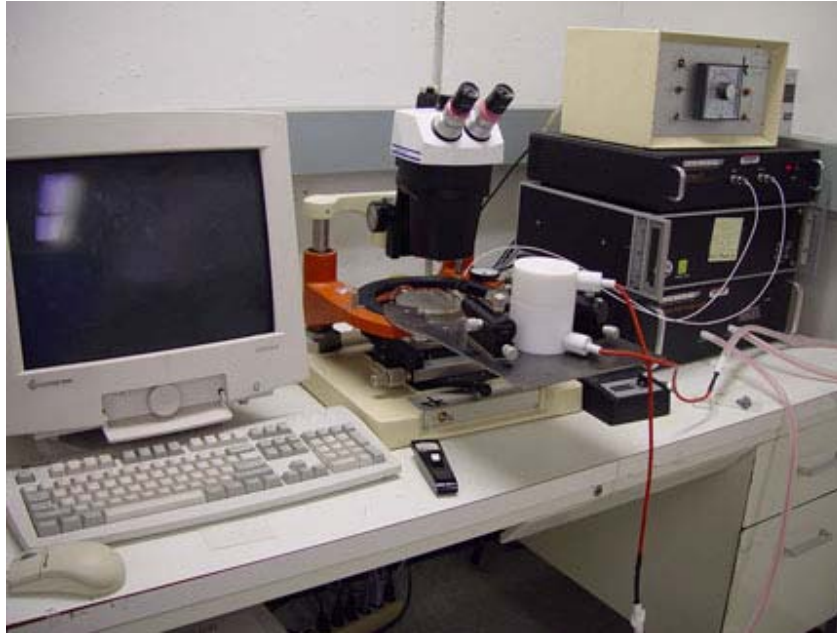
Figure 7.5. A picture of ferroelectric polarization measurement set-up at UMD.
