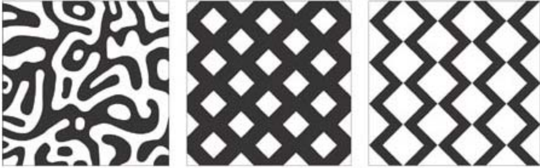
Figure 2.3: Typical spinodal decomposition showing well-defined periodicities and separated phases. 72
