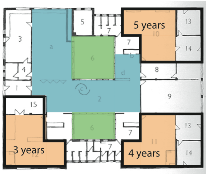
Figure 59 Classrooms at the corners of the building. The classroom entrances are connected to the piazza but acoustically and visually buffered by the cloakrooms. Stratton Treadway 2009.
