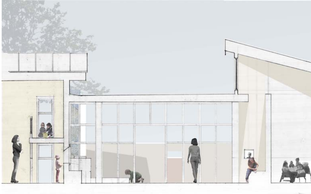
Figure 107 Section through the piazza space looking into the garden showing the way the butterfly roofs overlap the space and drain into the water pool and cistern. Stratton Treadway 2009.
