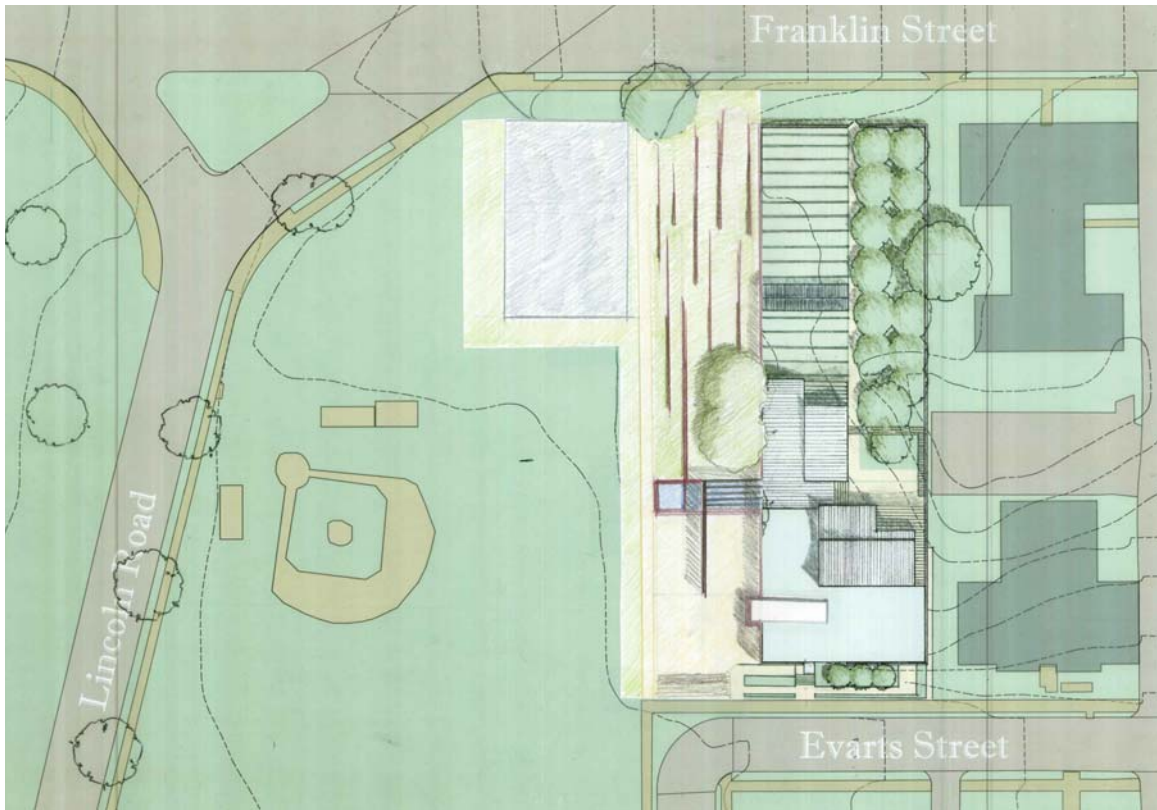
Figure 121 Revised site plan showing development of western landscape and new stair which engages the garden. Stratton Treadway 2009.
