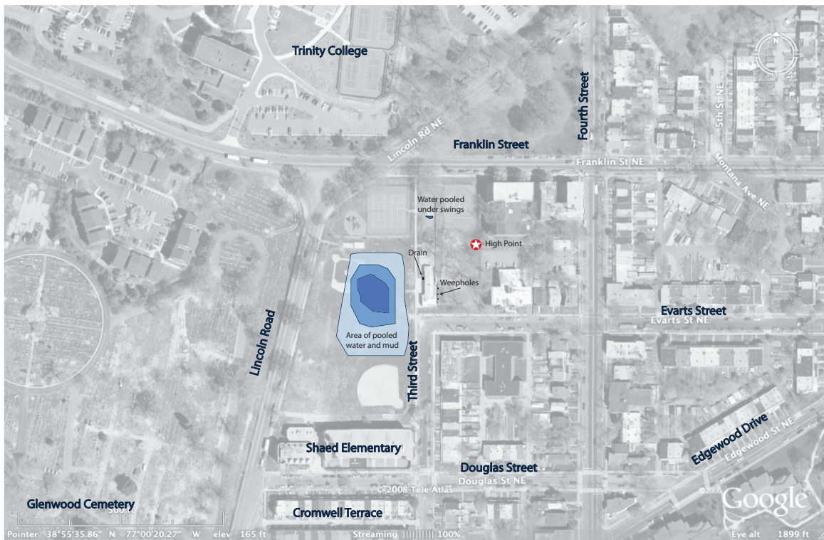
Figure 85 Water pools on the playing field after it rains and has no place to go. Stratton Treadway 2009.
