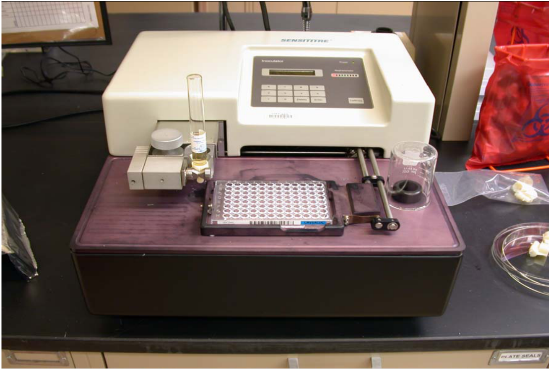
Figure 1: Photograph of Sensititre™ antimicrobial susceptibility testing system (Trek Diagnostic Systems, Westlake, Ohio)
