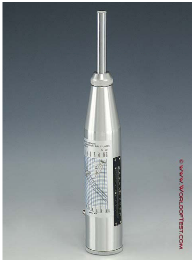
Figure 2-4: Use of the Rebound Hammer
