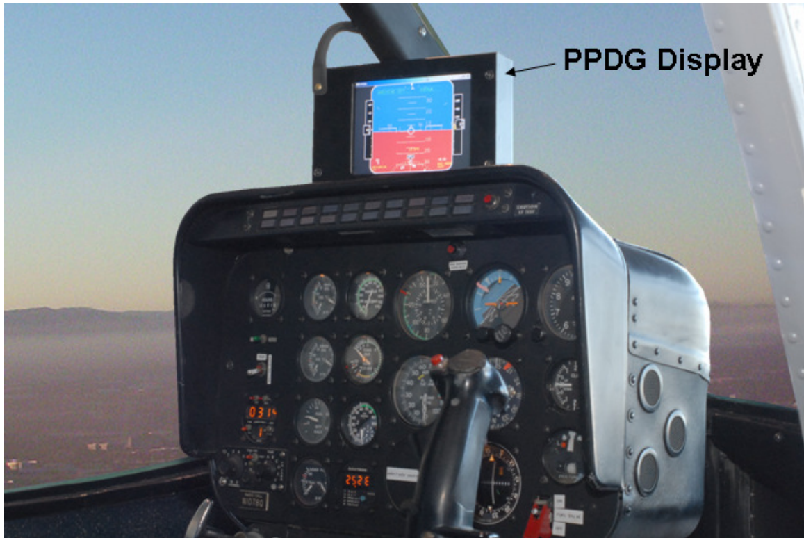
Figure 5.6: PPDG display mounted in cockpit.
