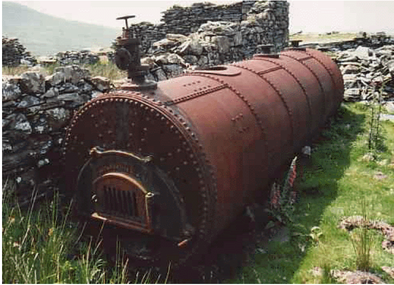
Figure 6. A Cornish boiler similar to those used aboard early American steamboats. The Cornish design had a single flue.
