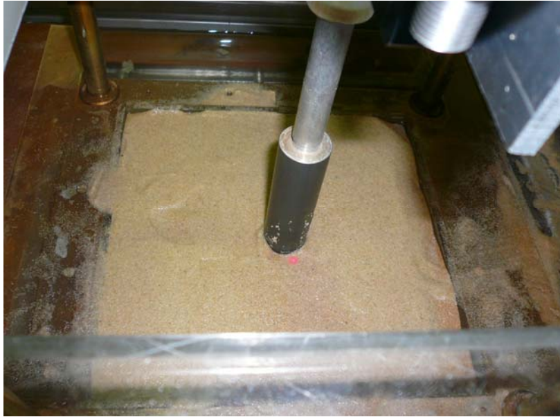
Figure 4.2 laser displacement sensor for the simulated earthquake shaking experiment.
