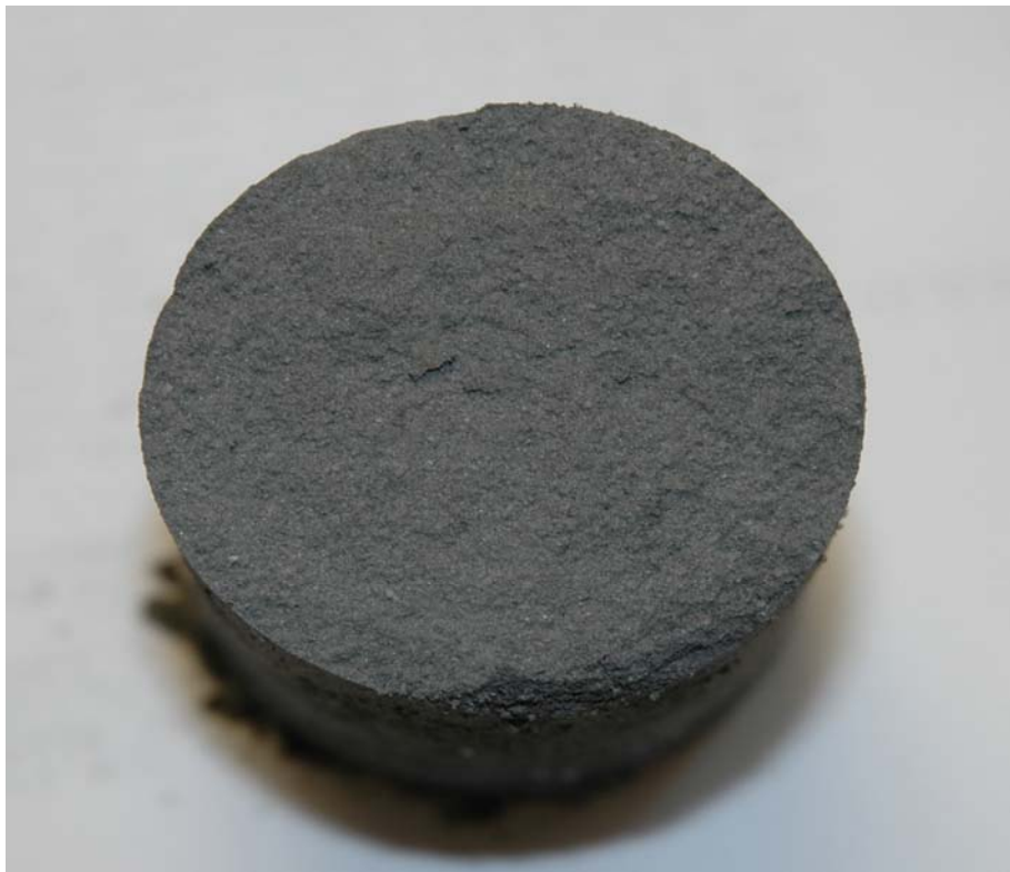
Figure 3. 5. Transversal section through the mixture layer of column specimens
