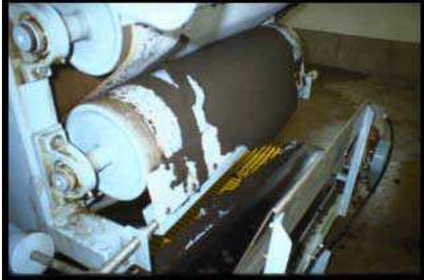
Figure 3.5: Dewatered solids cake dropping from belt filter press [59]
