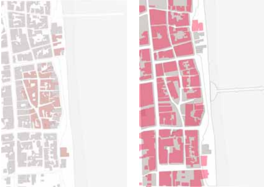
Fig.86. Figure ground of the site as it was in the first half of the 19 th century to the left while on the right, the proposed intervention (in red) superimposed on the old street layout. This demonstrates the attempt to retain traces of the old streets.
