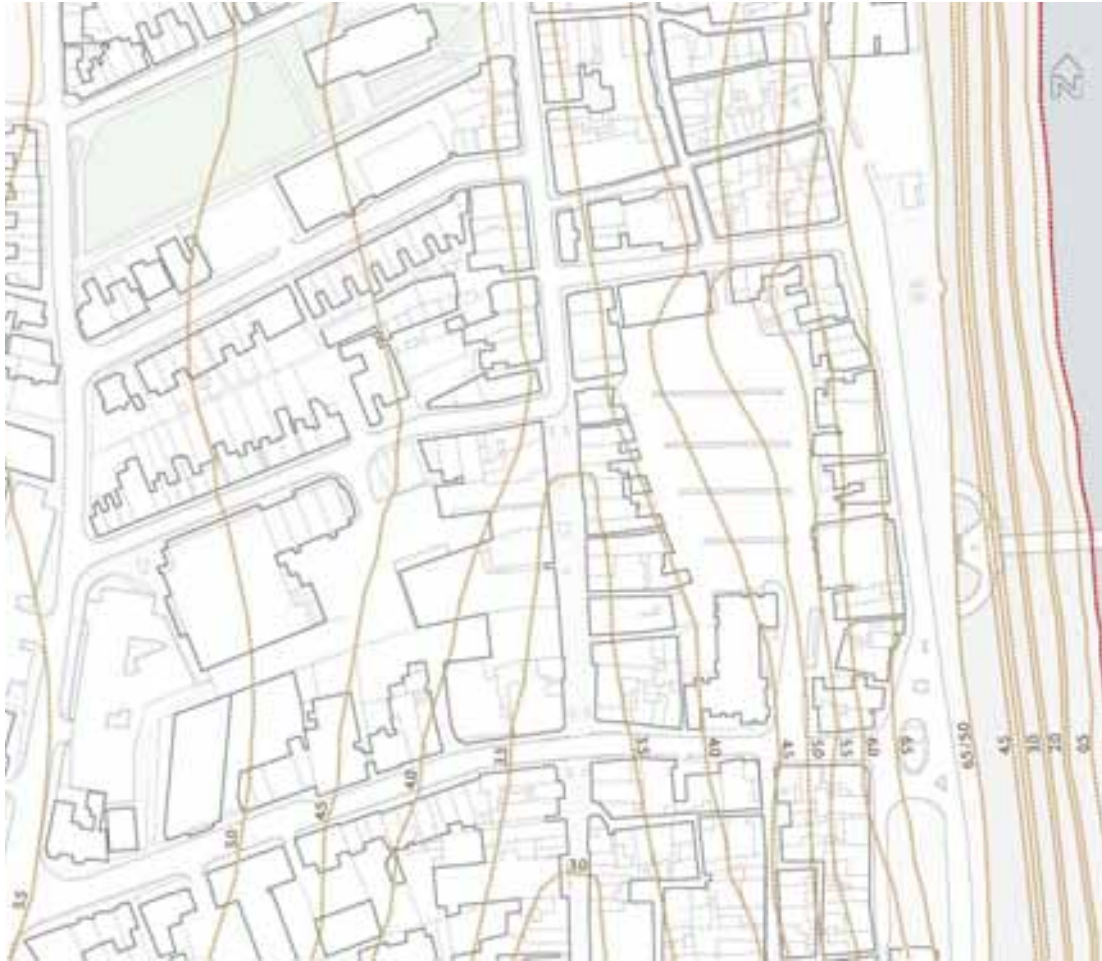
Fig.59. Topography: The promenade is on a ridge 6.5 meters above sea level, The High street is lower at around 3.2 meters. There is little change in elevation north- south
