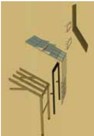
Fig.101. Exploded wall section showing glass enclosed by steel, enclosed by wood.
