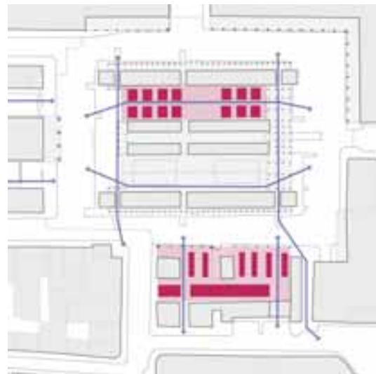
Fig.8. Defined by these bars, larger covered market areas are arranged along the secondary circulation paths. The overall sense is of a sequence of streets enabling access, reflecting the original need to maximize flow of goods and visitors
