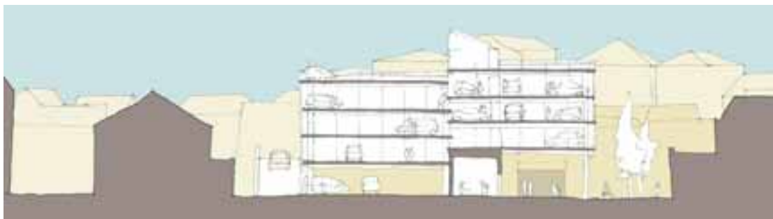
Fig.84. Section through car park, showing the staggered floor plates which help to maximise parking, as well as create a taller profile to the passage linking high street with the train station. Small retail units have been incorporated to line the 'passage'.
