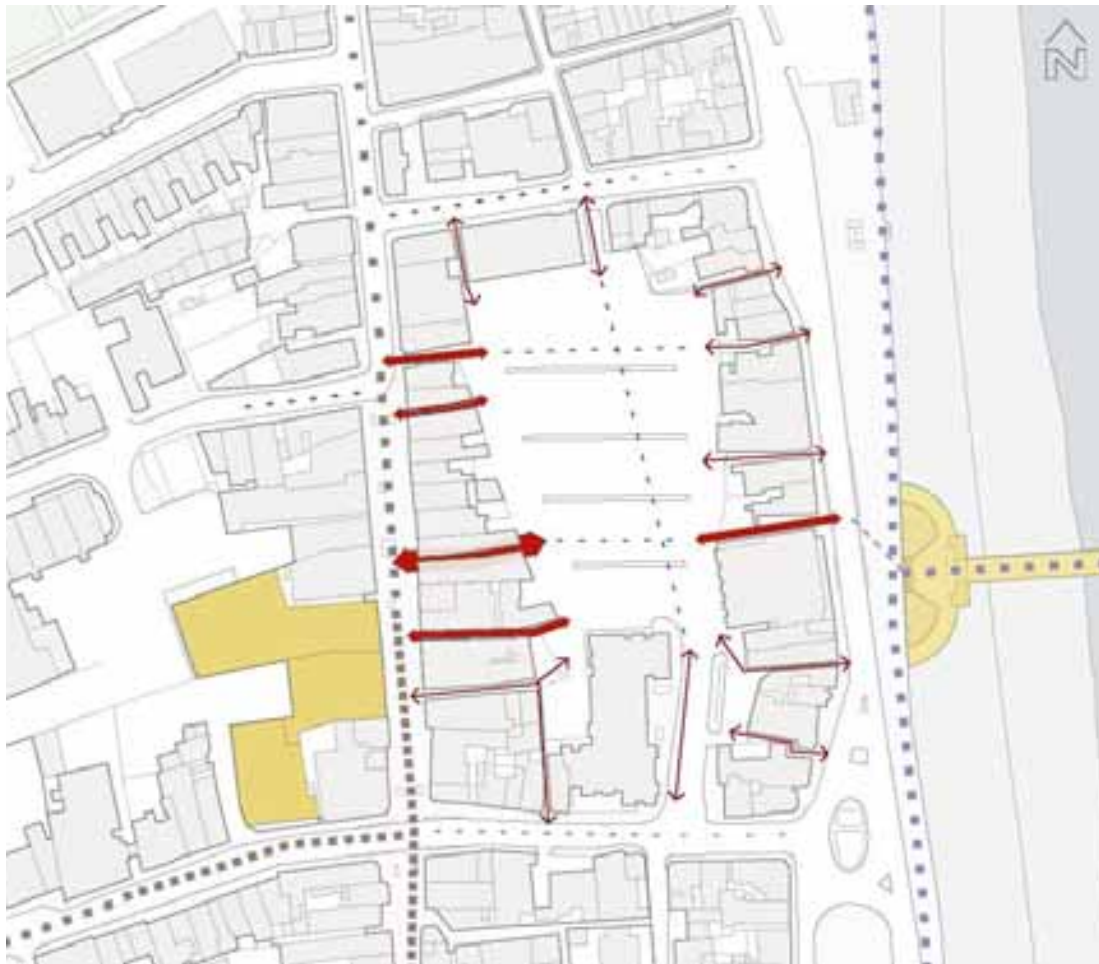
Fig.63. Pedestrian Circulation: access points to and from the site are numerous and are vestiges of the lanes that used to used to run across the site. The dotted lines show the density of pedestrian traffic around the site and illustrate the principal desire lines across the site. This main stores, marked in orange, that are the principal draws to the high street. The blued dotted line shows the promenade along the seafront and that there is little interaction between the foot traffic.
