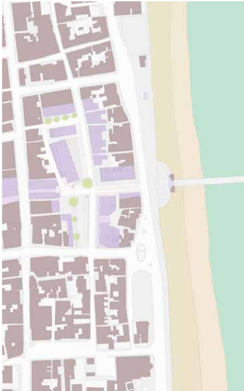
Fig.85. Site Plan: The relocated library lines the east edge of a market square, while a new institutional/office building, defines the north side of the new link between the pier and the site. The market house occupies space to the north of the site while the street edge of middle street is maintained by new residential/commercial properties.
