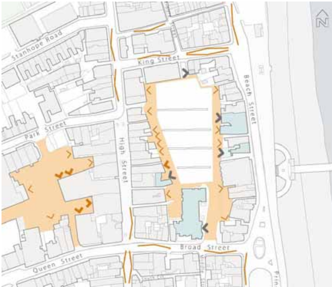
Fig.62. Service Access: The area to the west behind the high street is only used for service access while the site itself mixes customer parking with service. The edges of the car park act as service access for the surrounding commercial uses. Other surrounding commercial premises only serviced from the street. The buildings in blue are accessed by the public directly from the site.
