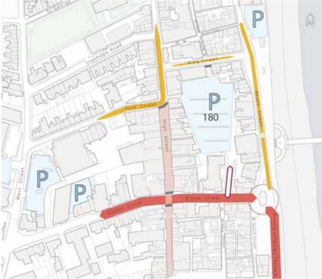
Fig.61. Vehicular Circulation: the principal roads meet at a nearby roundabout on the sea front. The only vehicular access into the site is from Broad Street. The High Street is pedestrian at this point (shown in pink).
