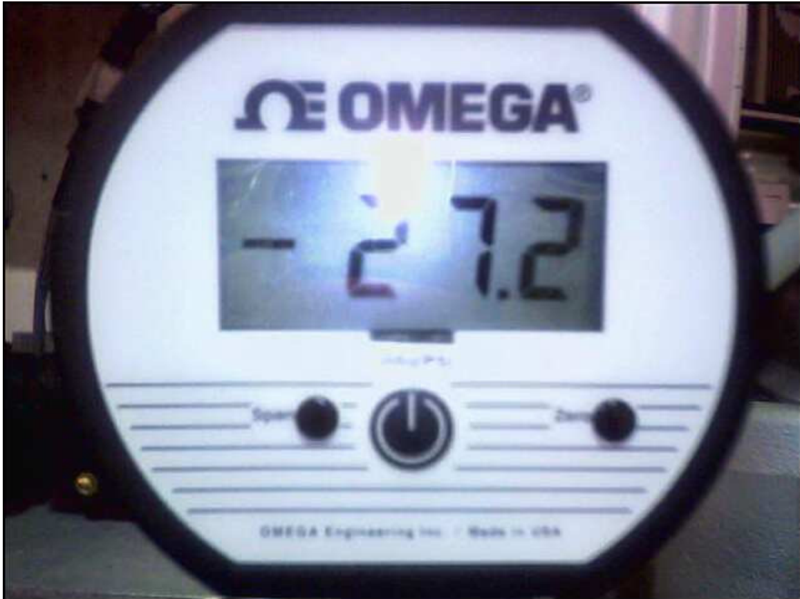
Fig. 3.10. Picture of pressure sensor showing pressure less than 27.0 in of Hg in vacuum (0.1 atm)
