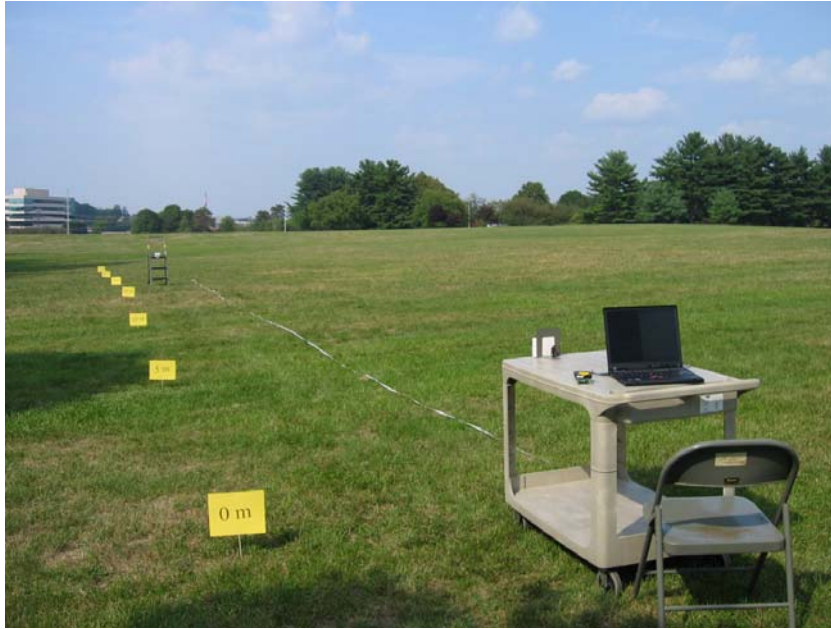
Figure 5.23: Configuration of setup for distance estimation test
