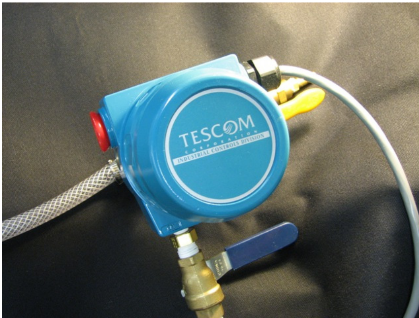
Figure 2-7: TESCOM ER3000-SV1 Electronic Pressure Controller used in the experimental setup
