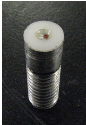
Figure 2-13: Mask stub used during release agent spraying
