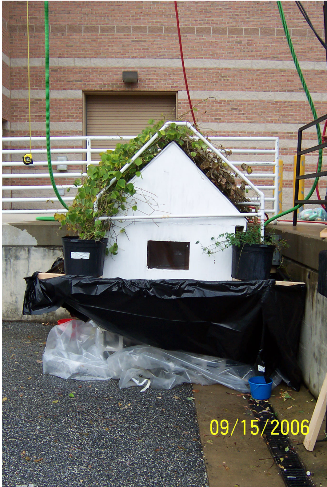
Figure 5.8. Cloak, house, and gutter system under rainfall simulator.
