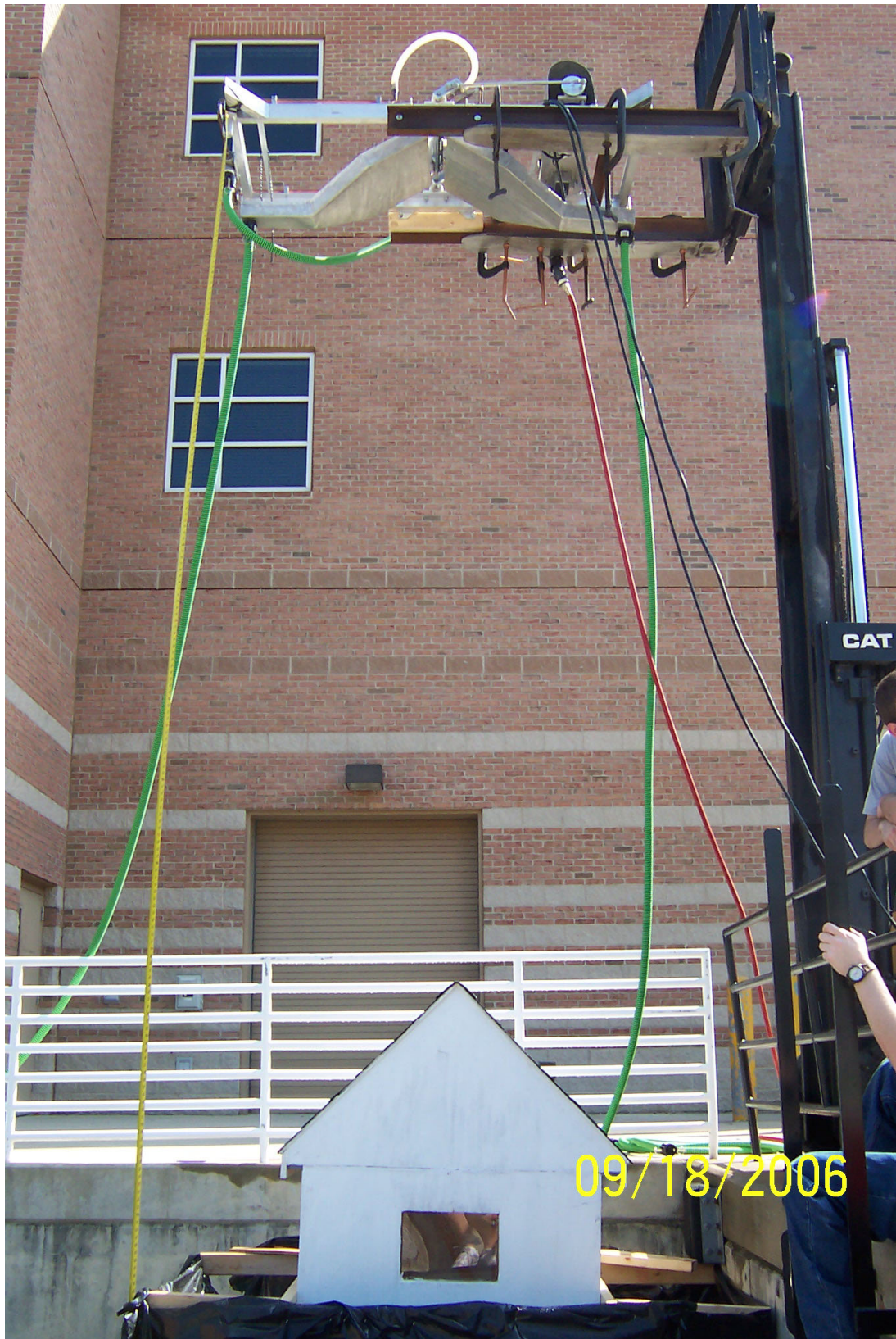
Figure 5.9. Rainfall simulator shown in place above model house.
