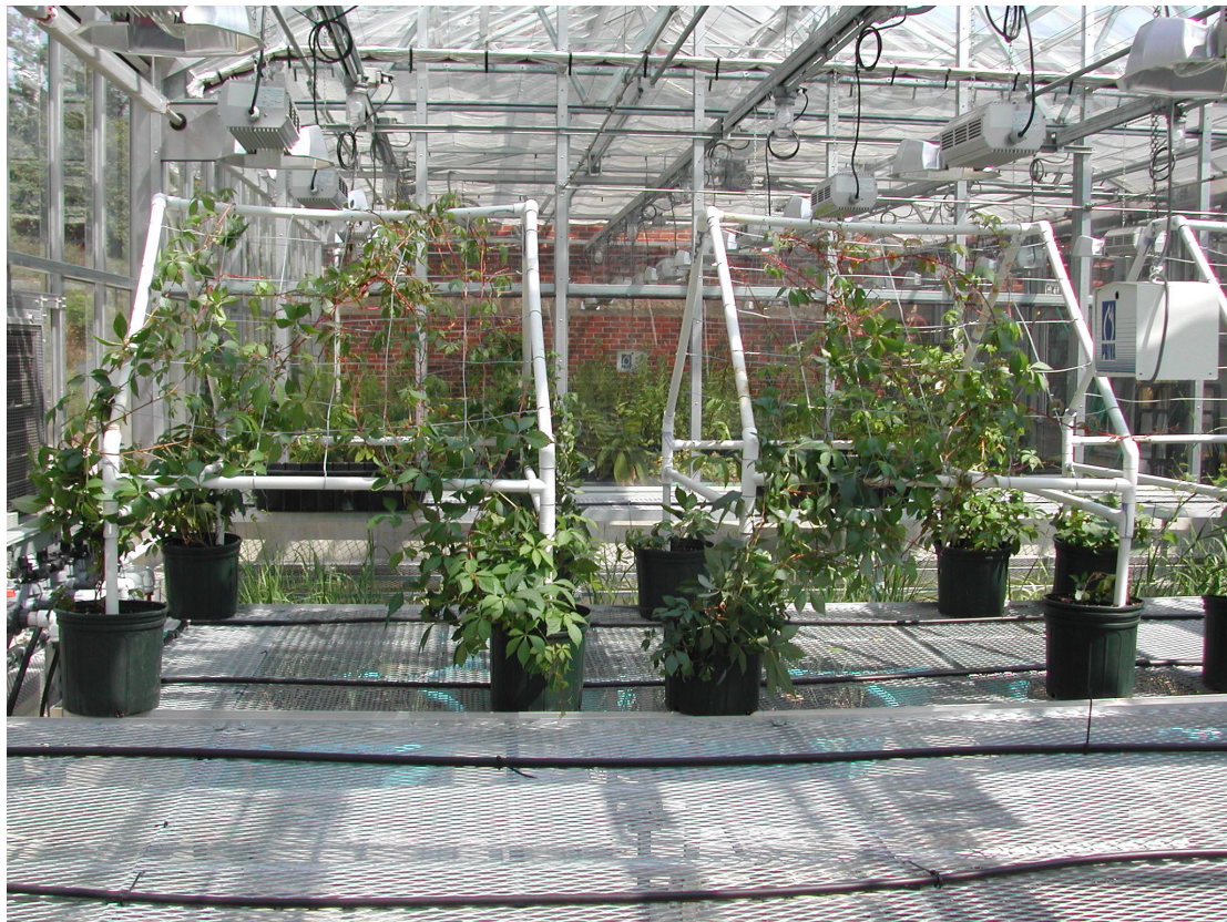
Figure 3.2. Green cloak composed of PVC frames, wire trellis mesh, and potted vines.
