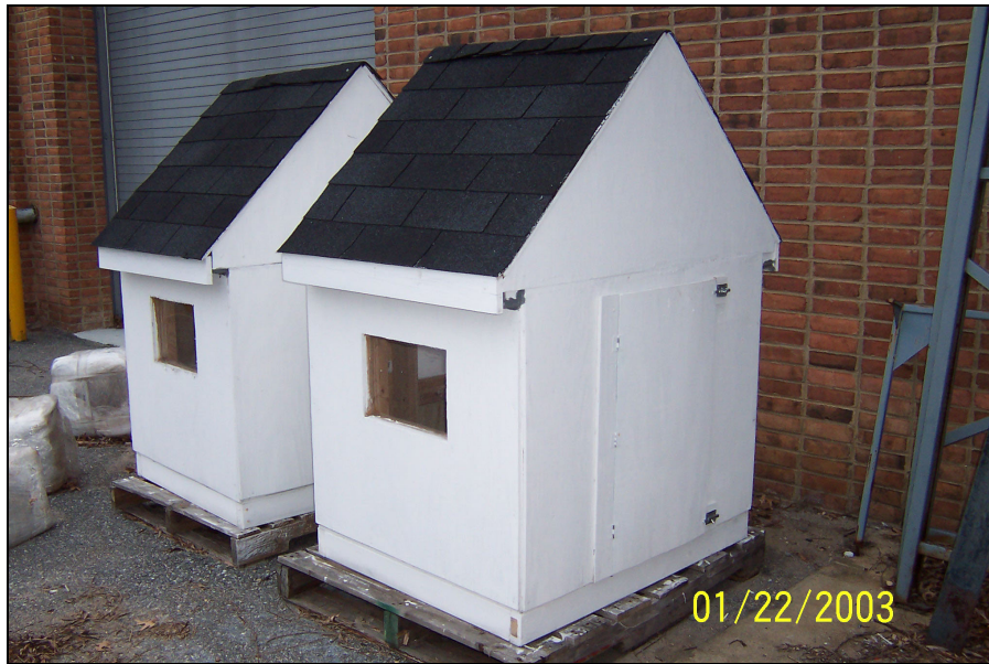
Figure 3. Scaled, wood-frame, plywood-covered model buildings used during heat and runoff experiments with the green cloak.
