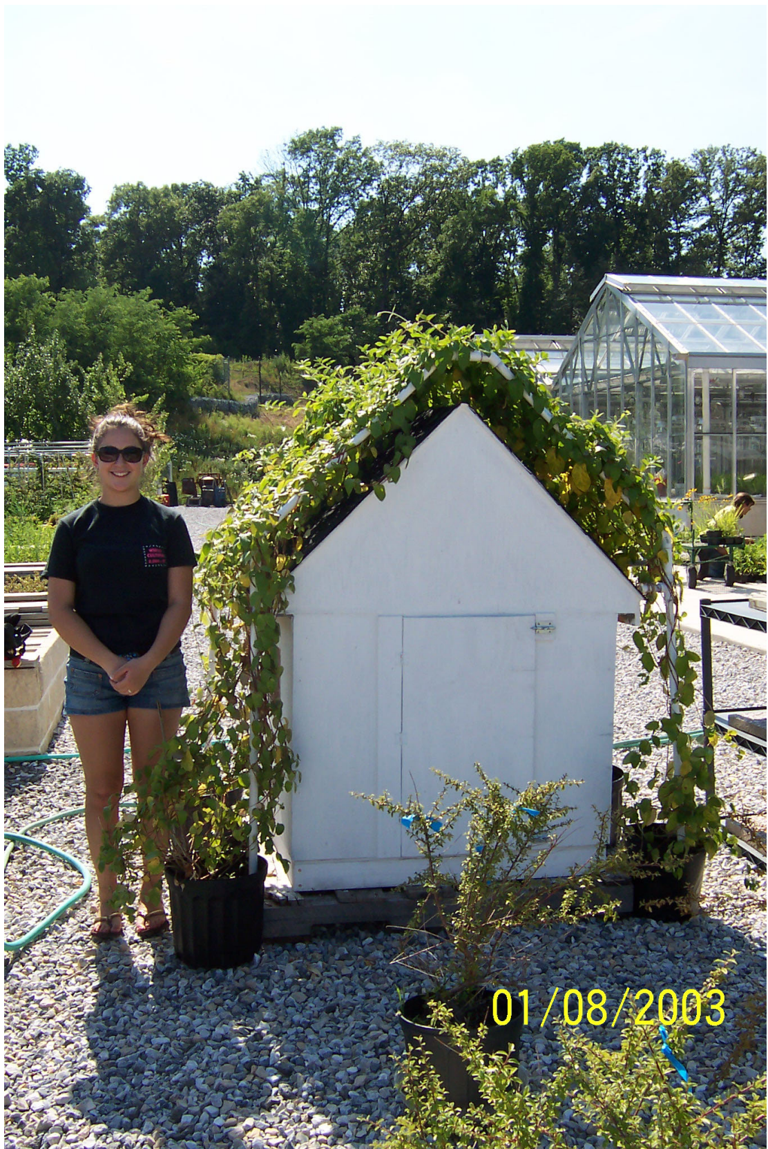
Figure 5.5. Green cloak fit over model house with 20 cm gap.
