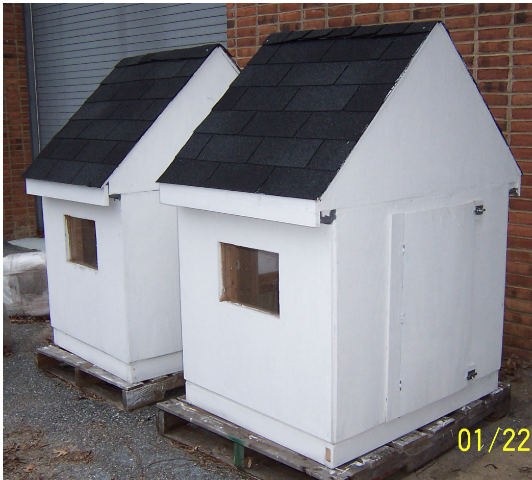
Figure 3.1. Scaled model plywood houses with shingled roof.
