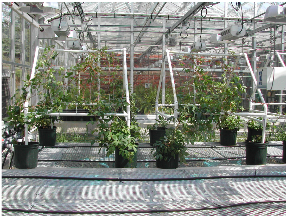
Figure 5.4. Green cloak composed of PVC frames, wire trellis mesh, and potted vines.
