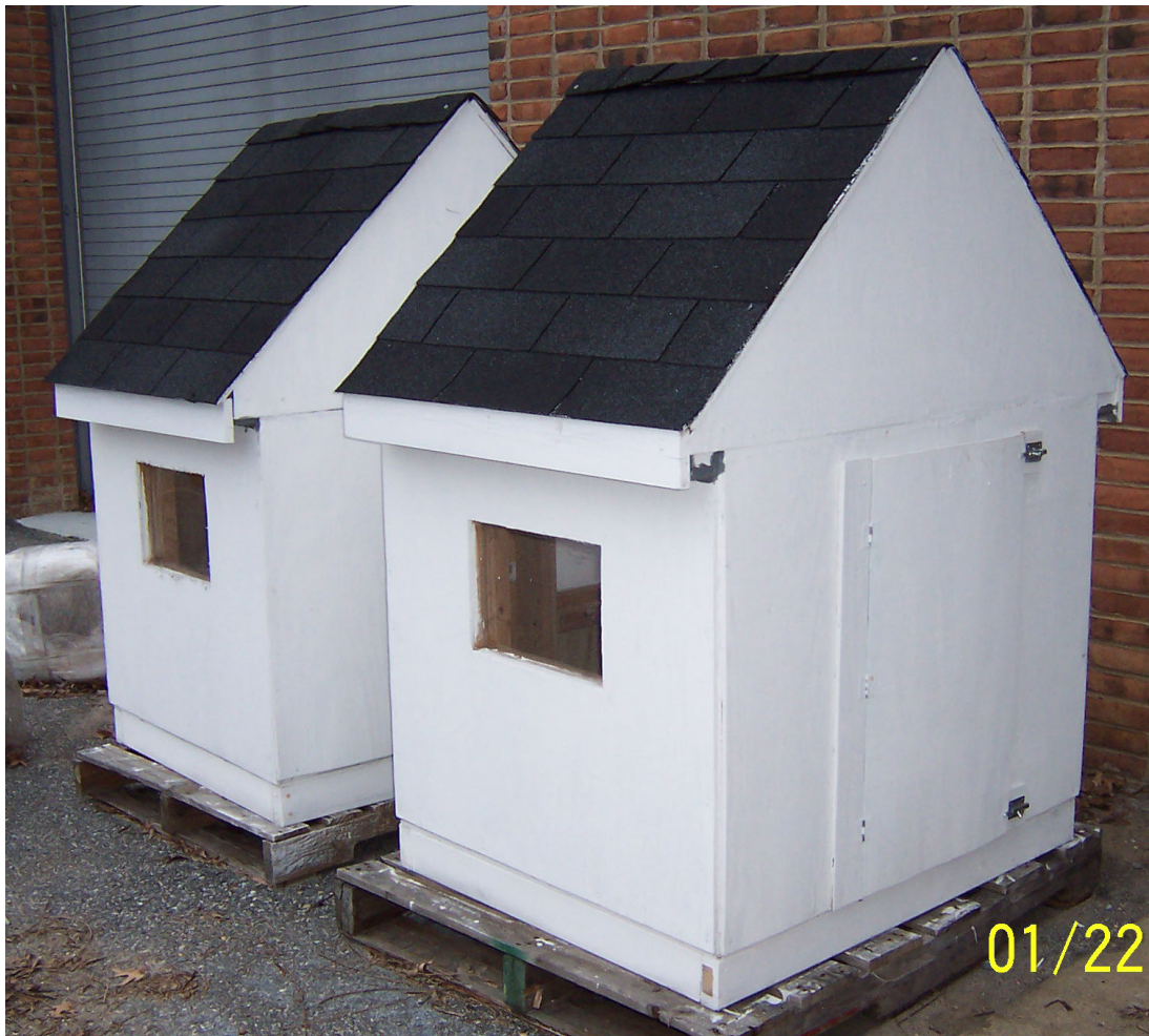
Figure 5.2. Scaled model plywood houses with shingled roof. We used only one house in the rainfall experiment.
