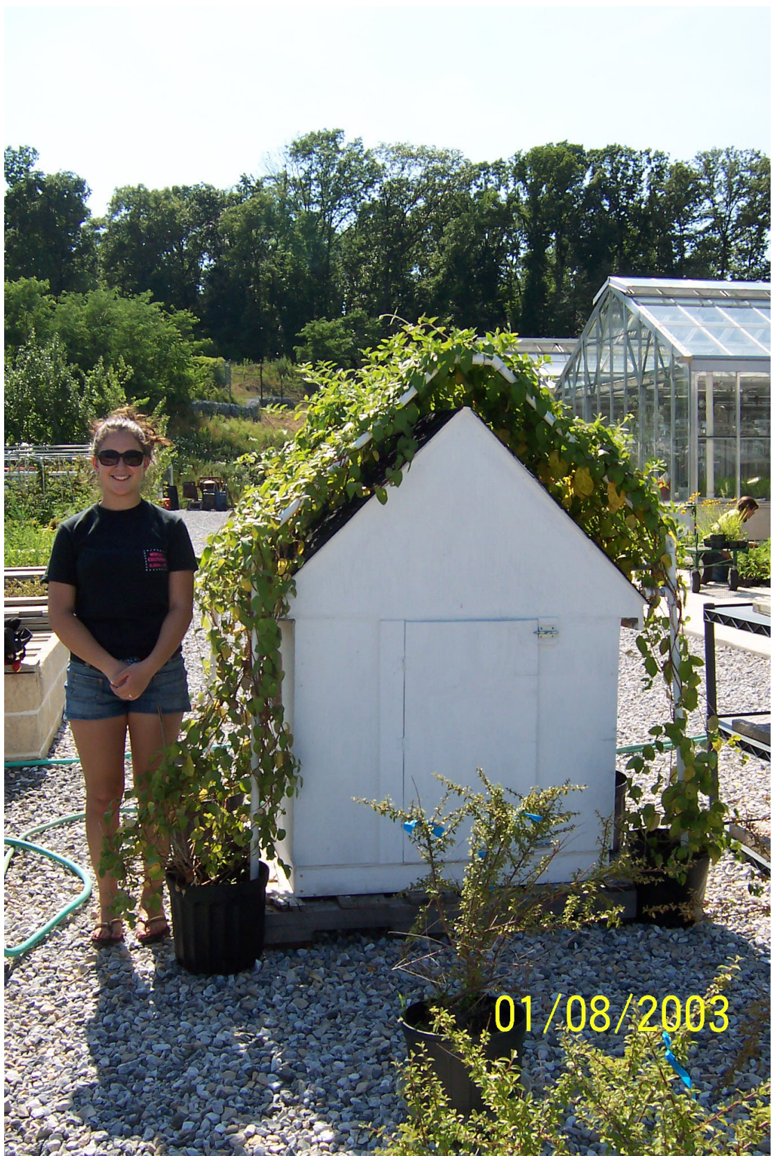
Figure 3.3. Green cloak fit over model house with 20 cm gap.
