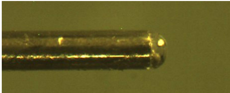
Figure 4.6: Photograph of the deterioration of the sputtered layer after in-tail testing.
