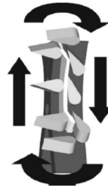
Figure 9: The path that the follower makes as it travels around the guide.
