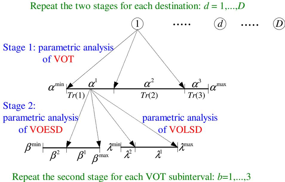
Figure 6.2 Sequential Parametric Analysis Method
