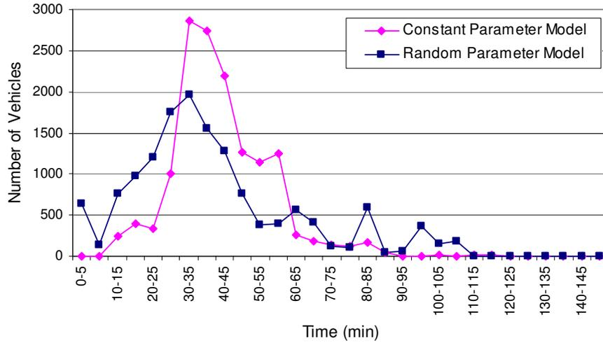
Figure 6.11 Comparison of departure patterns in constant and random parameter models on the test network
