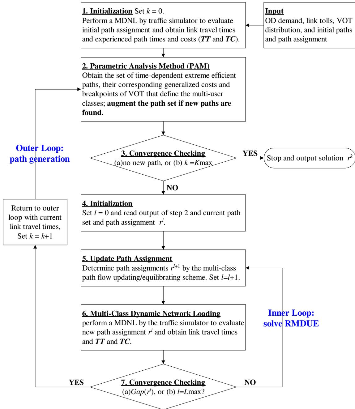
Figure 4.1 Flow chart of the BDUE solution algorithm
