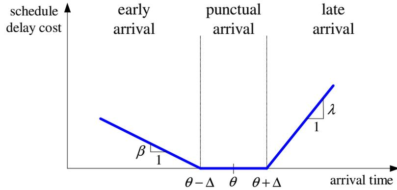
Figure 2.3 The piece-wise linear function of schedule delay cost
