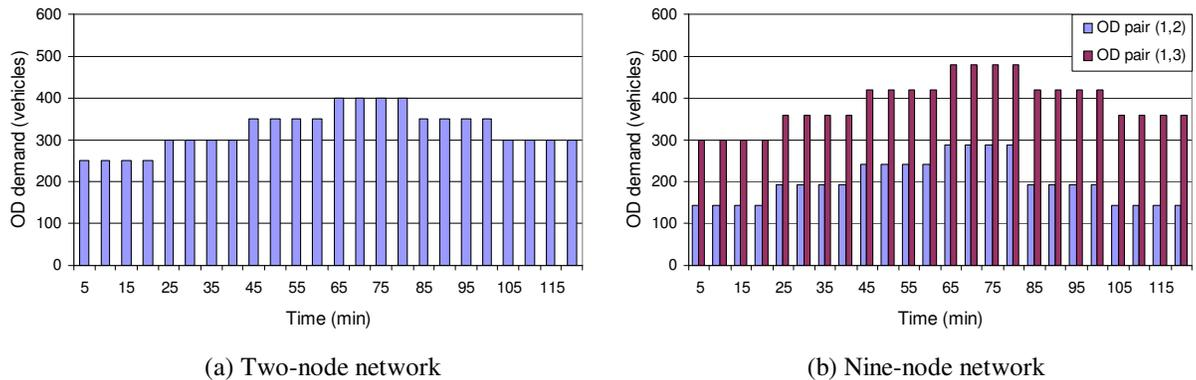
Figure 3.4 The time-dependent OD demands of the two small networks
