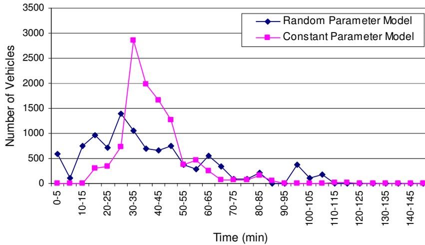
Figure 6.12 Comparison of time-varying toll road usage in constant and random parameter models on the test network
