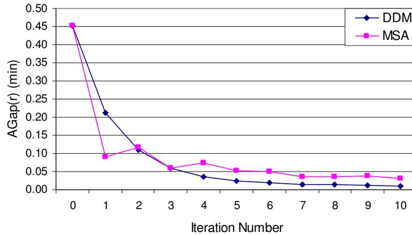
Figure 3.5 Convergence patterns of DDM and MSA on the two-node network
