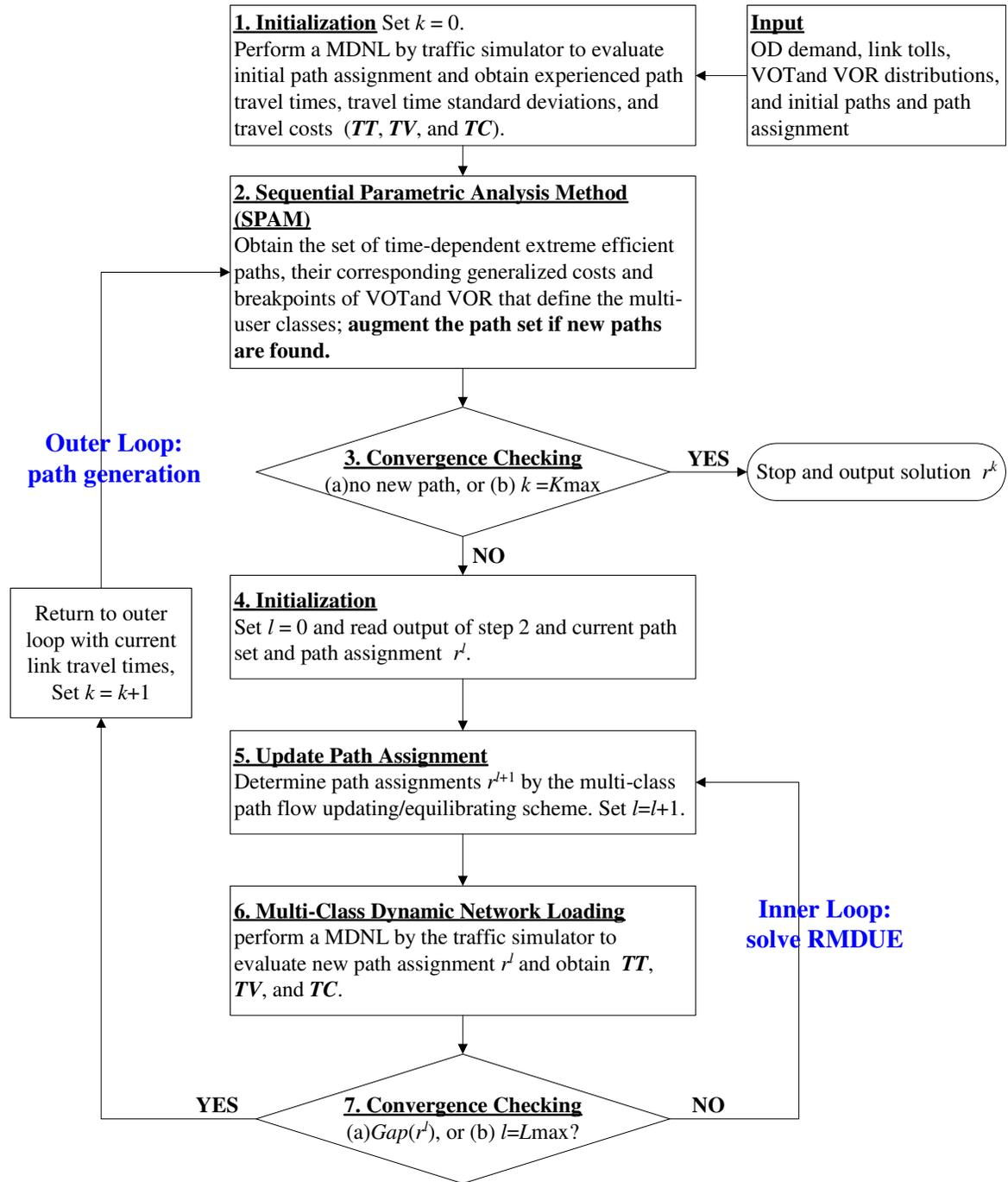
Figure 5.1 Flow chart of the MDUE solution algorithm
