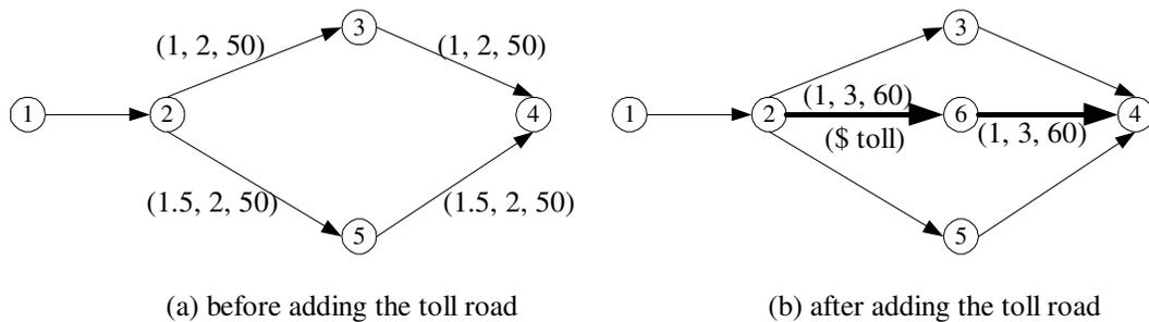
Figure 4.11 Before and after adding the toll road in a small test network
