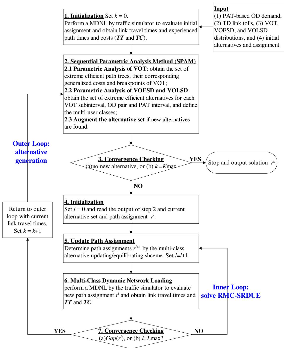
Figure 6.1 Flow chart of the MSRDU solution algorithm
