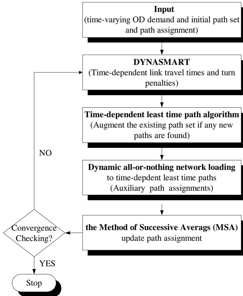
Figure 2.1 The simulation-based UEDTA algorithm by Peeta (1994)
