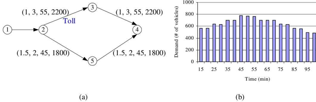
Figure 4.7 The small test network and time-varying OD demand
