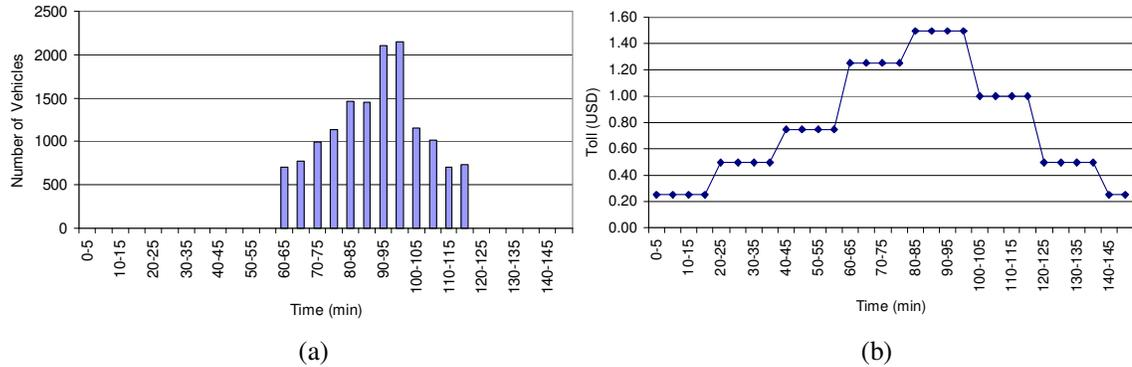
Figure 6.7 PAT distribution (a) and dynamic pricing scenario (b) in the test network
