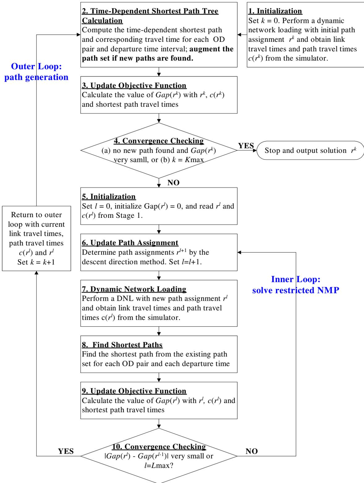
Figure 3.1 The column generation-based DUE algorithm
