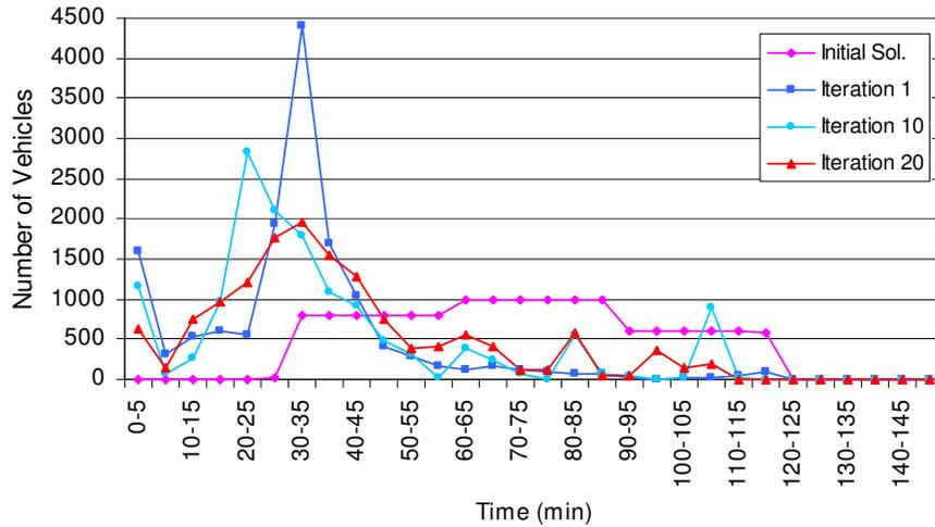
Figure 6.10 Convergence pattern in terms of departure time distribution on the test network
