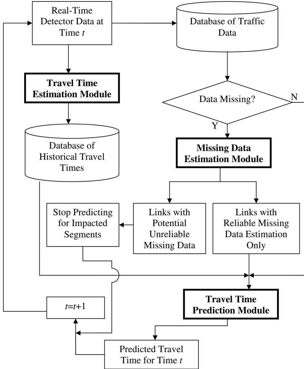
**Figure 3-2** System operational flowchart for the real-time operation stage
