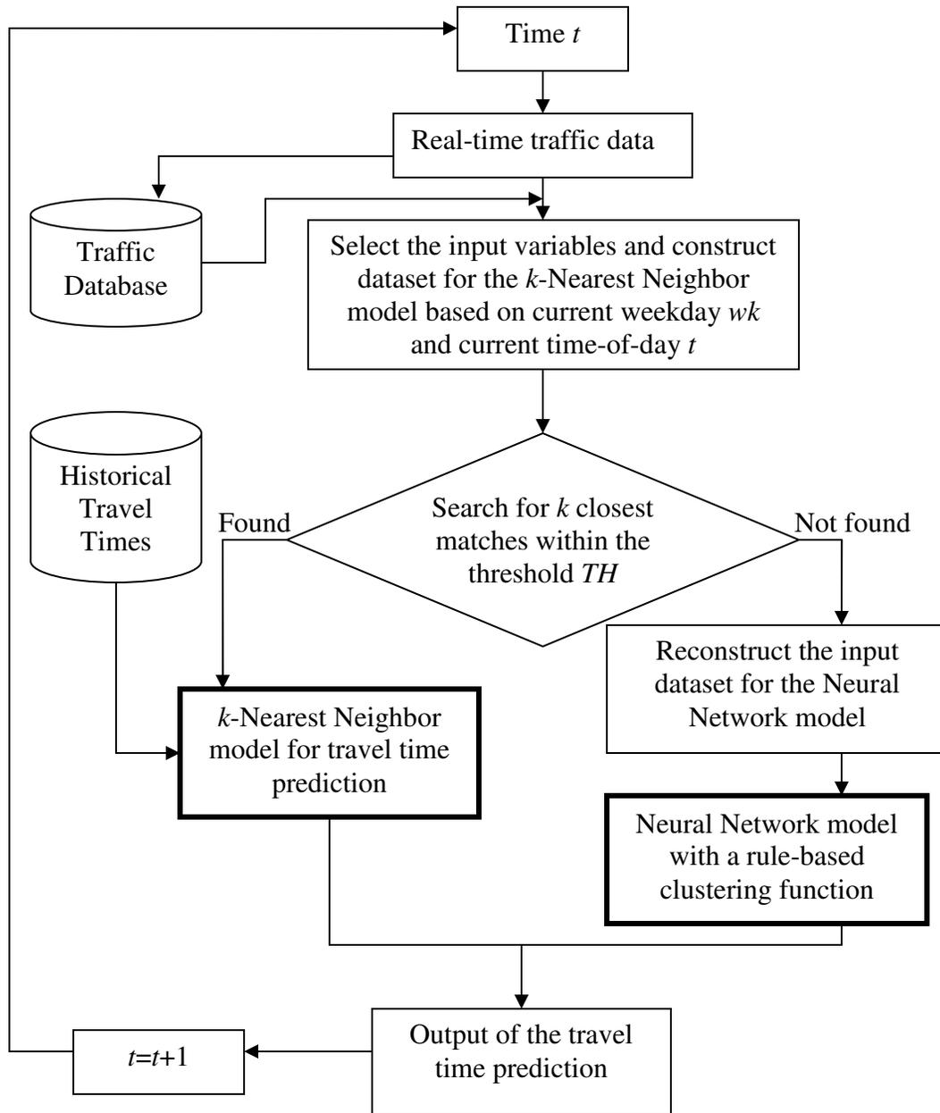
**Figure 5-1** Flowchart of the hybrid travel time prediction model
