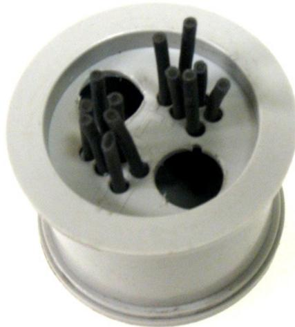
**Figure 24: Raw contacts in the mold**
