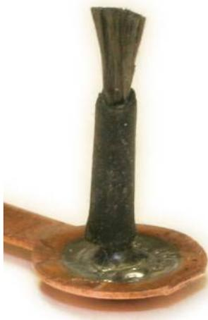
**Figure 15: A carbon fiber solder joint**
