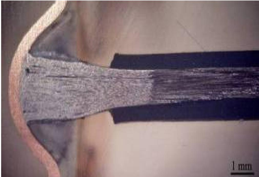
**Figure 16: Cross section of a carbon fiber solder joint**
