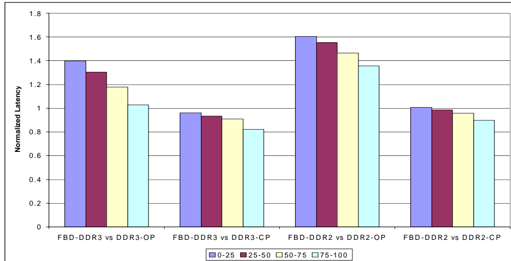
Figure 4.23. FBD vs. DDRx: Latency Improvements for different row buffer management policies. The figure shows the change in read latency achieved by a FBD system over its corresponding DDRx system as a function of workload bandwidth utilization for different row buffer management policies. The bandwidth utilization classification is done using the observed bandwidth for the corresponding DDRx system. Note that the latency improvements are plotted as normalized against the latency of a DDRx system. Latency averages are calculated for all workloads studied and all configurations run.
