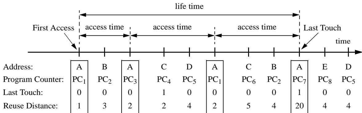
**Figure 1. A memory address trace, and various information associated with the trace used to predict last touch and/or reuse distance. Information includes memory addresses, memory reference program counters, last touch history, and reuse distance. Access and live times are indicated for a sequence of references to the memory address *A*.**
