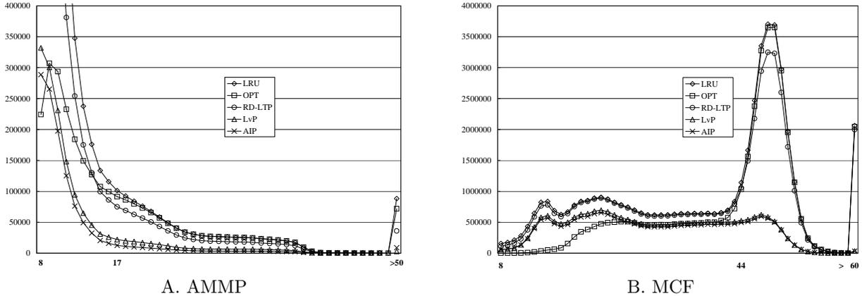
Figure 5. Last touch reference histograms under LRU, OPT, LvP, AIP, and RD-LTP cache management for the A. AMMP and B. MCF benchmarks. CRD = 17 and 44 for AMMP and MCF, respectively.
