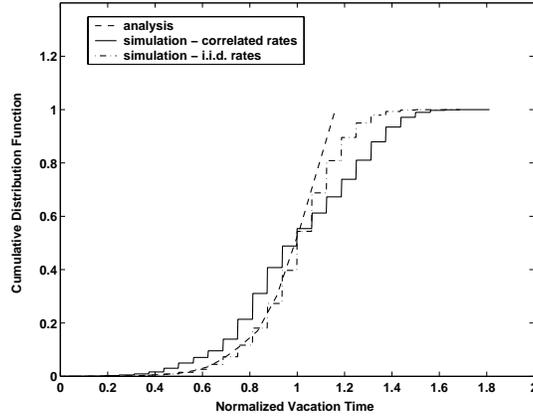
Fig. 8. Comparison of Vacation Time CDFs for  $\alpha = 50$  when channel rates are i.i.d. and correlated across time slots
