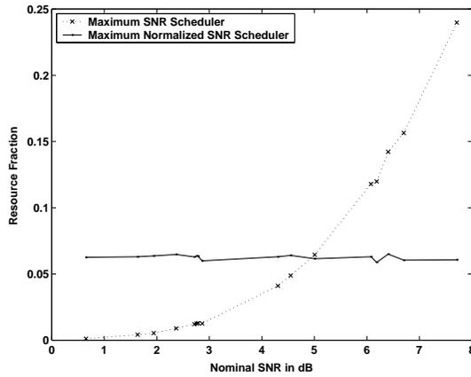
Fig. 9. Resource Fraction for 16 users at different nominal SNRs but identical channel statistics
