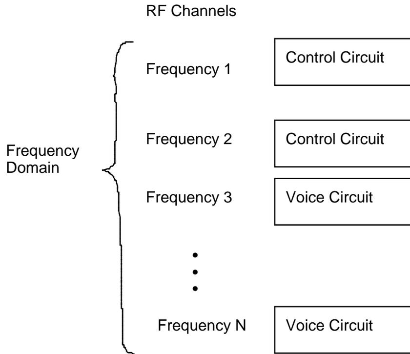
**Figure 4. FDMA Cellular System Architecture**
