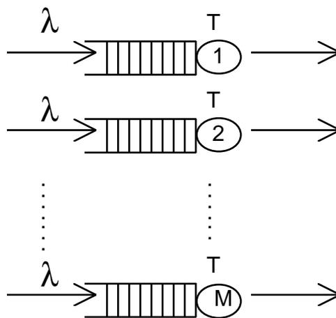
**Figure 15. FDMA Satellite System Architecture**
