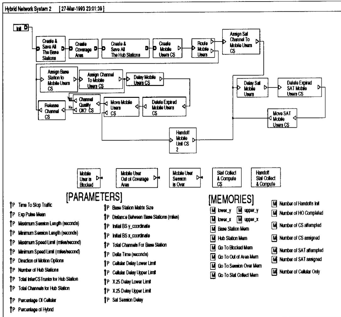
Figure 19. Hybrid Network System Model
