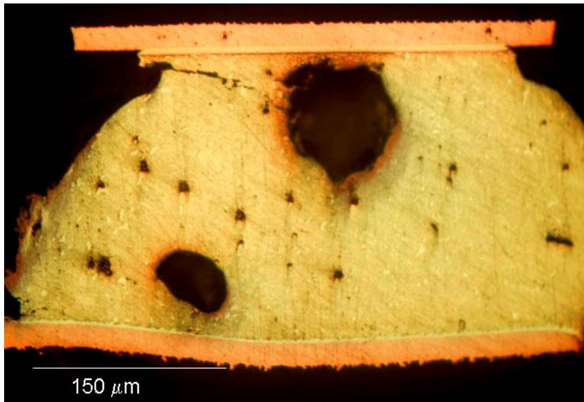
Figure 2-20: Relatively big voids located in the middle of damage path
