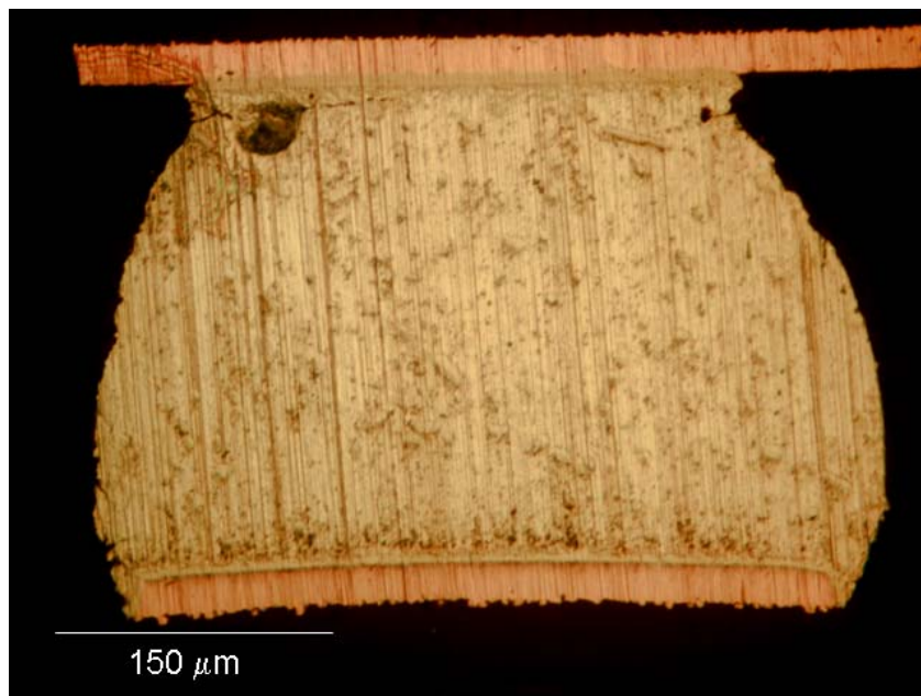
Figure 2-21: Small void located close to damage initiation site
