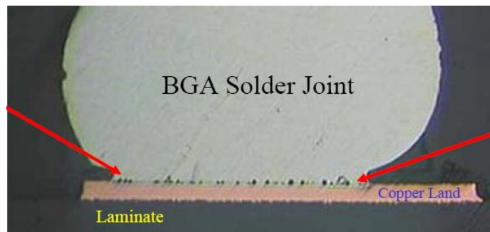
Figure 1-10: planar micro voids at the interface of solder and PCB pad [Aspandiar, 2005]
