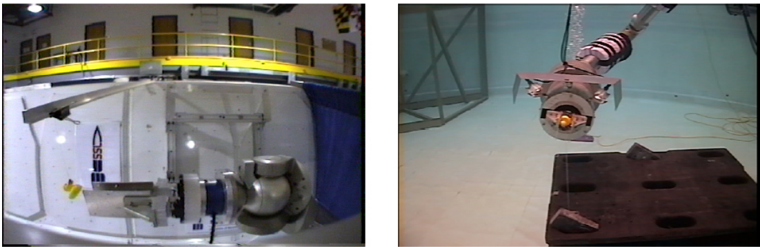
Figure 6-2: Ranger successfully grabbing a target in both testing environments
