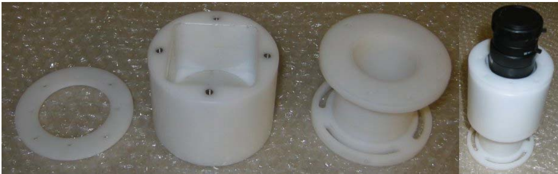
Figure 5-3: Internal Camera Mount Assembled and Disassembled
