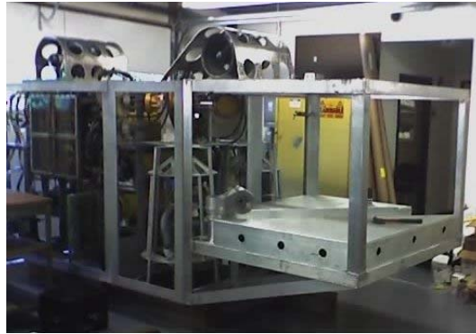
Figure 5-4: SSL Manipulator Test Frame Attached to WHOI Sled
