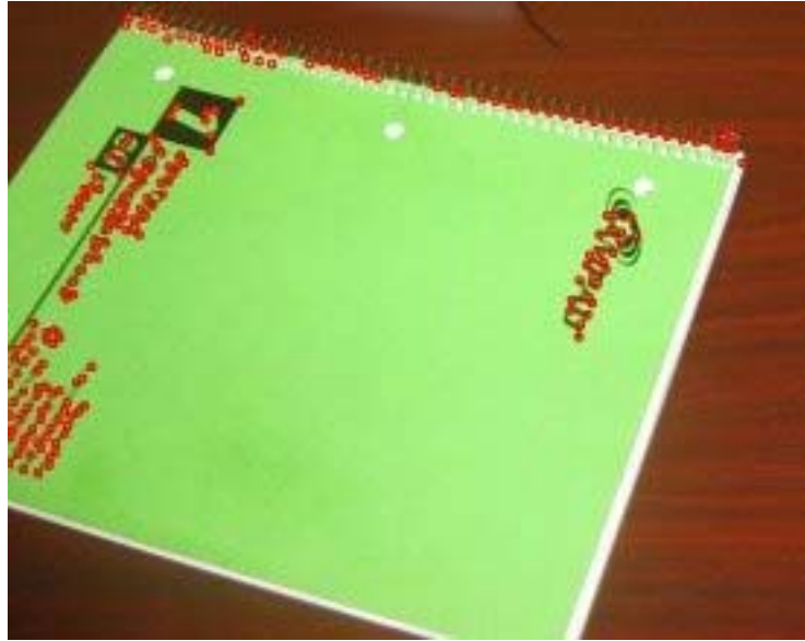
Figure 2-6: Output from OpenCV corner detection algorithm
