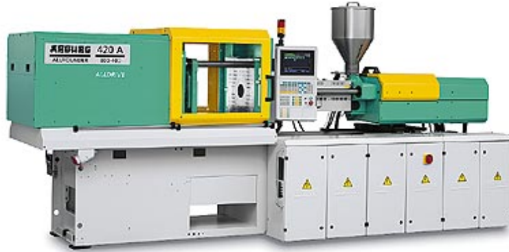
Figure 1.3: Photo of a typical injection molding machine Source: http://www.arburg.com/english/products/po_a0001.htm
