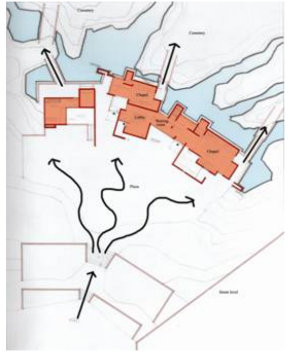
Figure 50- Site plan showing the approach to the chapels. Buildings act as visual retaining wall keeping the view to the cemetery until the visitor is at the chapels.
