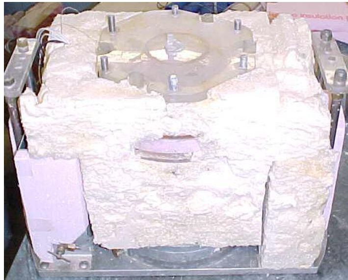
Figure 3. 1 Insulated model container before placement in circular bucket
