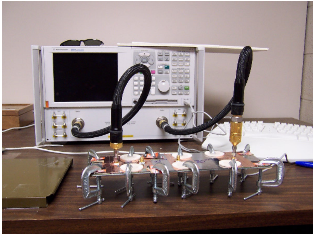
Figure 2-4 Measurement setup using a Vector Network Analyzer (VNA). S_{21} is a representative for transfer impedance between port 1 and port 2.
