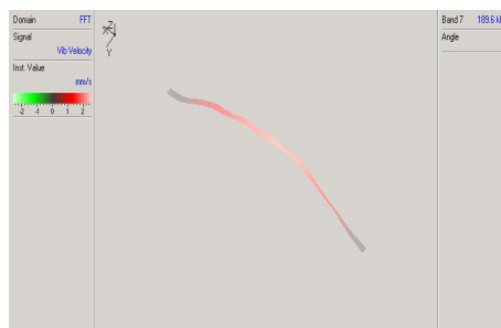
Figure 9.10 Measured mode shape at frequency 3 from Figure 9.9.
