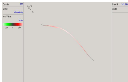
Figure 8.33 Measured mode shape at frequency 3 from Figure 8.31.
