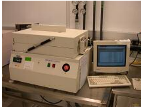
Figure 4.1 Tencor FLX-2908 system used for wafer bow and stress measurements.
